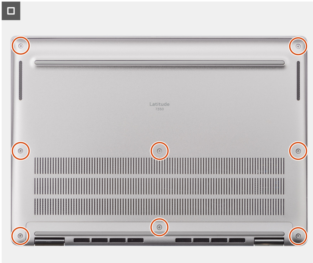
Figure 20. Installing the base cover
