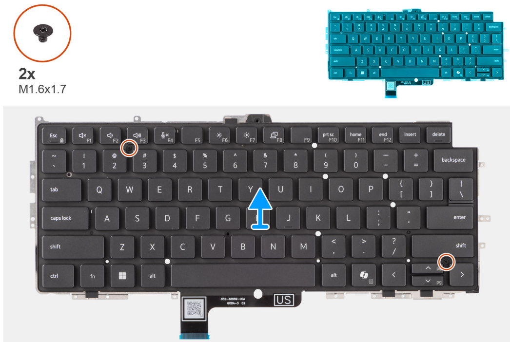
Figure 79. Removing the keyboard
