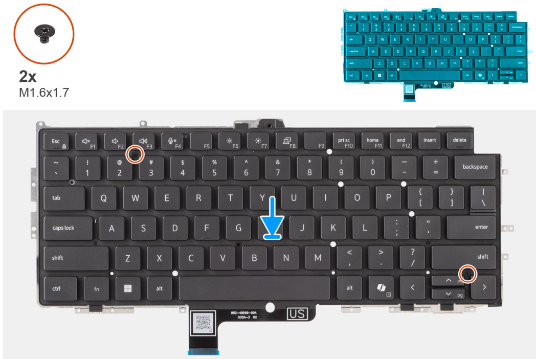
Figure 82. Installing the keyboard
