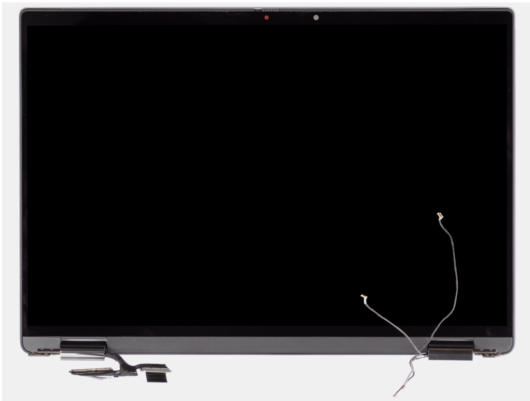
Figure 51. Display assembly with WWAN-antenna cables
