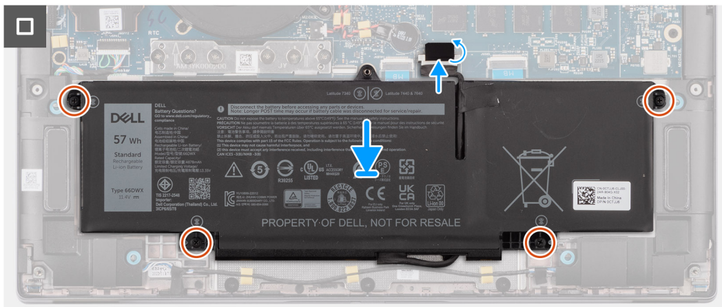
Figure 43. Installing the 3-cell battery
