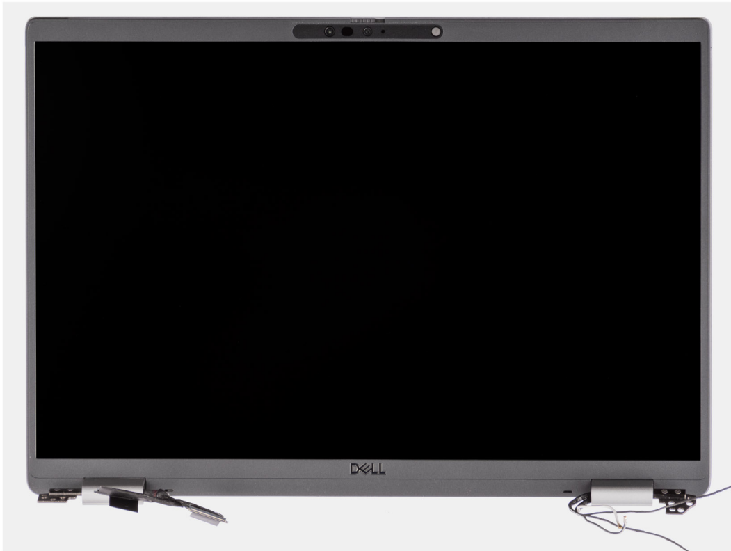
Figure 52. Display assembly with WWAN-antenna cables
