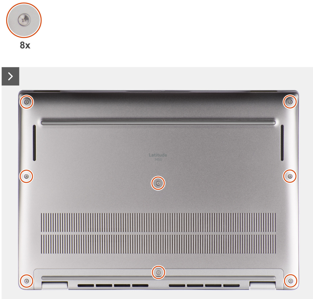
Figure 16. Removing the base cover
