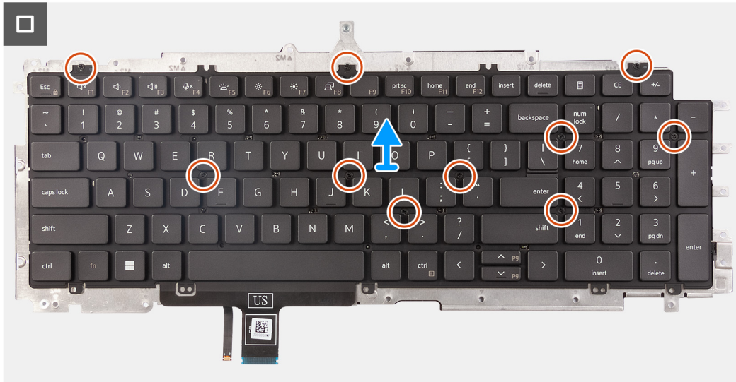
Figure 66. Removing the keyboard
