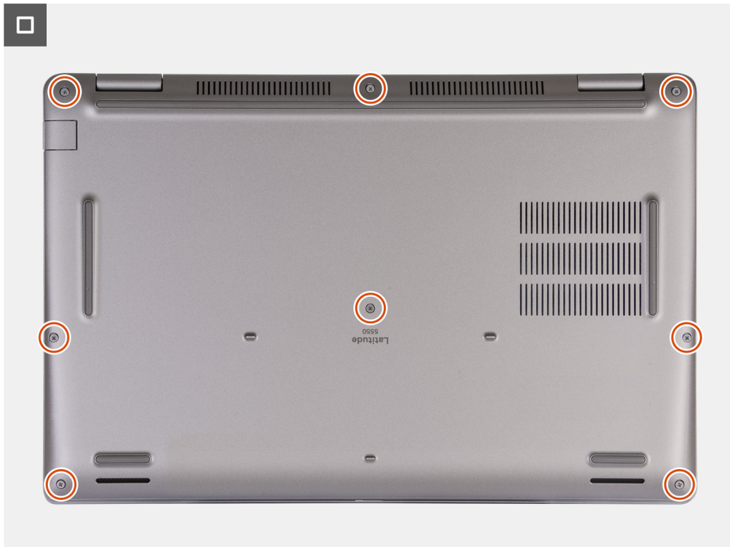
Figure 18. Tighten the captive screws
