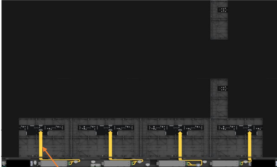
4X Column Power Cables
