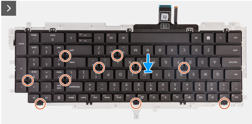
Figure 71. Installing the keyboard
