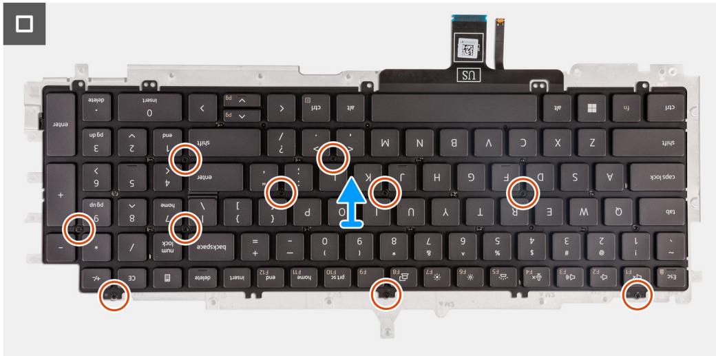
Figure 70. Removing the keyboard
