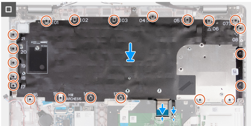
Figure 72. Installing the keyboard
