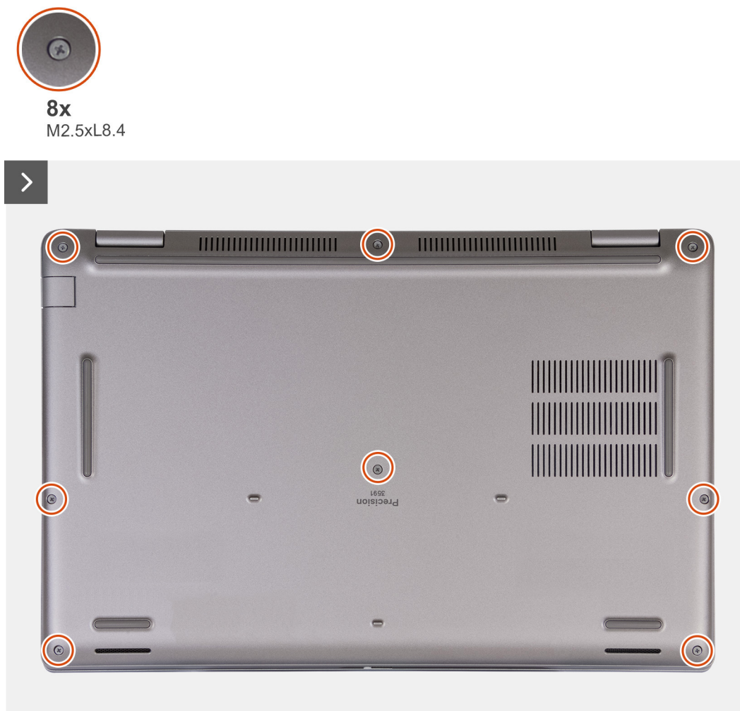
Figure 13. Loosen the captive screws
