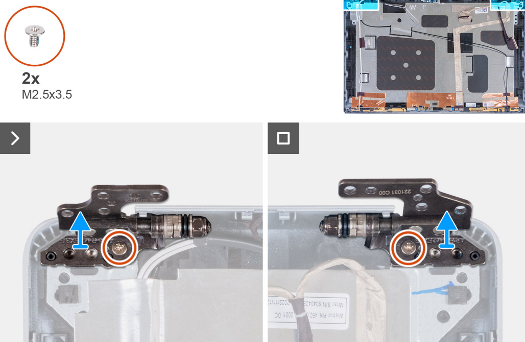
Figure 90. Removing the display hinges
