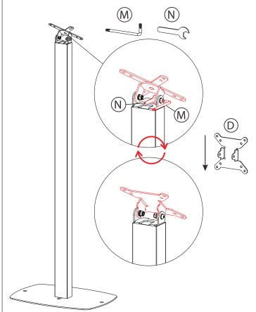
2A. Using the allen key tool and wrench tool (M &N), remove the existing screws on the X VESA. Then put on the new vesa bracket (D) and reapply screws and washers. The new bracket will be compatible with the VESA charging station.
