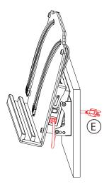
1D. When cable routing in the wall mount installation, take the power cord provided (E) and route one end through the rear bracket area into the charging station device as illustrated. Take the other end and either route it through the opening on the wall or down the wall into the outlet depending on what kind of setup you have.
