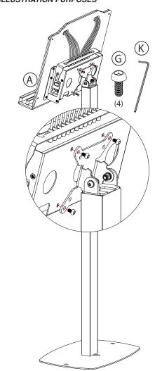
2B. Repeat Step 1C to initially setup the back bracket with the charging station. Then align the VESA holes of the back bracket with the VESA bracket. Using provided tool (K), rotate in 4 screws (G) until securely fastened.
