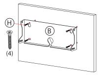
1A. When mounting directly into the wall first align bracket to the wall. Use 4 screws (H) and rotate in with screwdriver (not included) at the 4 corner openings until securely fastened.
