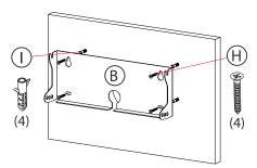
1B. When mounting using anchors, first predrill the wall at the mounting locations. Insert the anchors. Align the wall brackets and rotate in 4 screws (H) using a screwdriver (not included until securely fastened.
