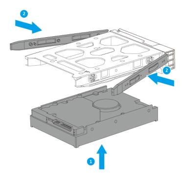
**d.** Attach the screws to further secure the drive.
