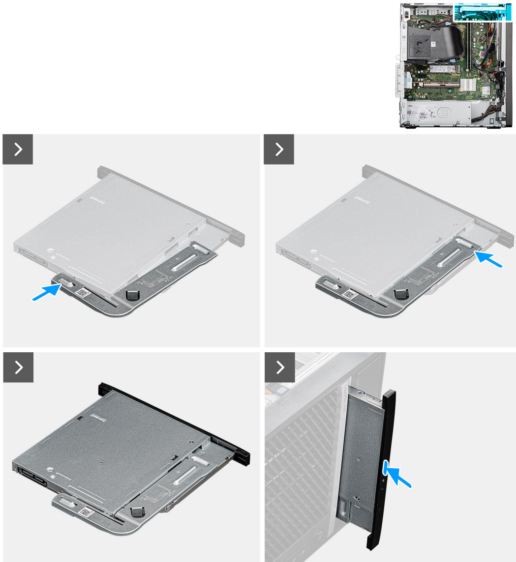
Figure 39. Installing the slim optical drive
