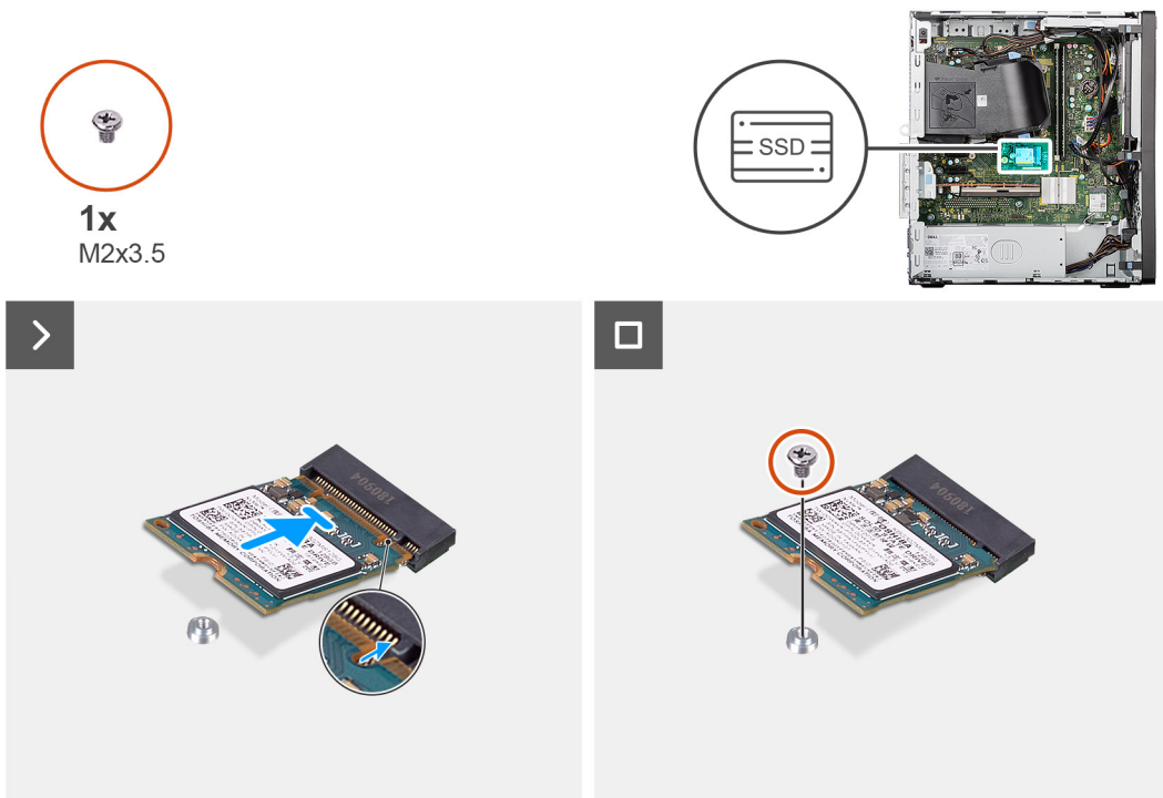
Figure 21. Installing the M.2 2230 solid-state drive
