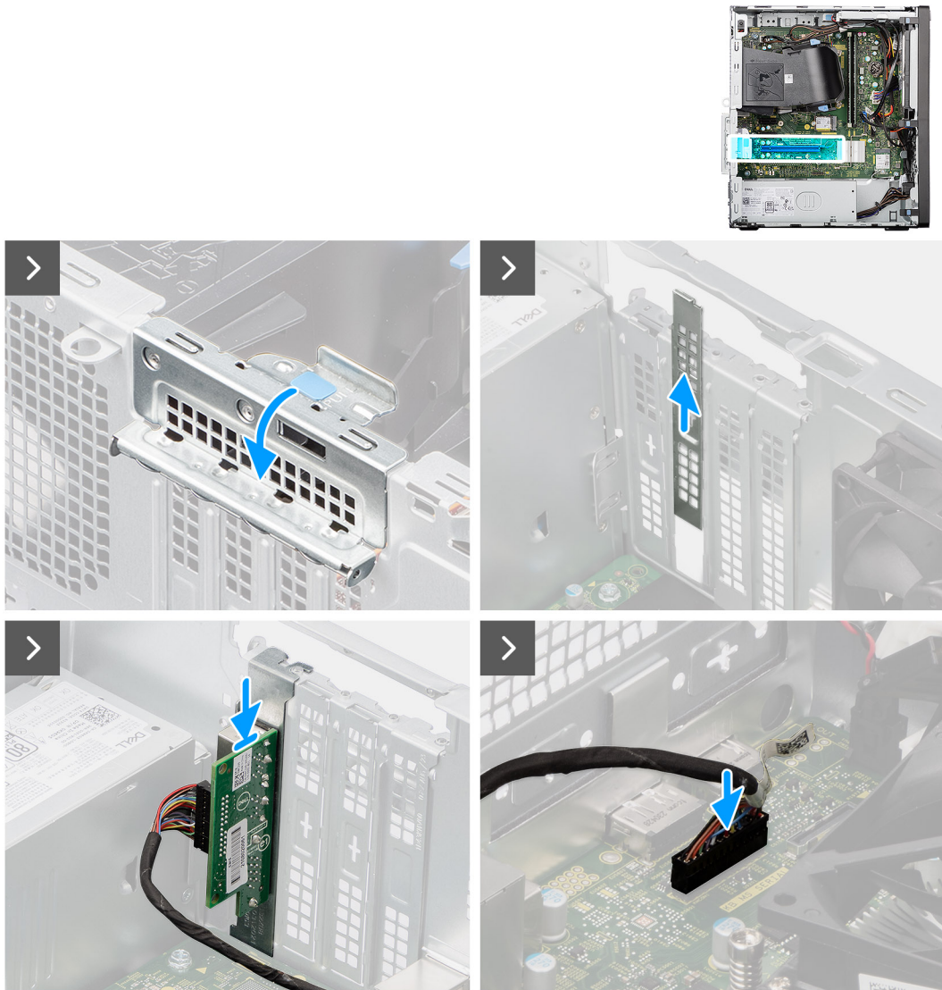
Figure 74. Installing the optional PS2 and serial module
