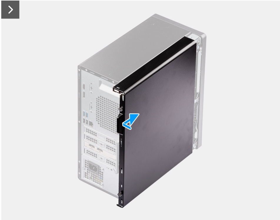
Figure 11. Installing the side cover
