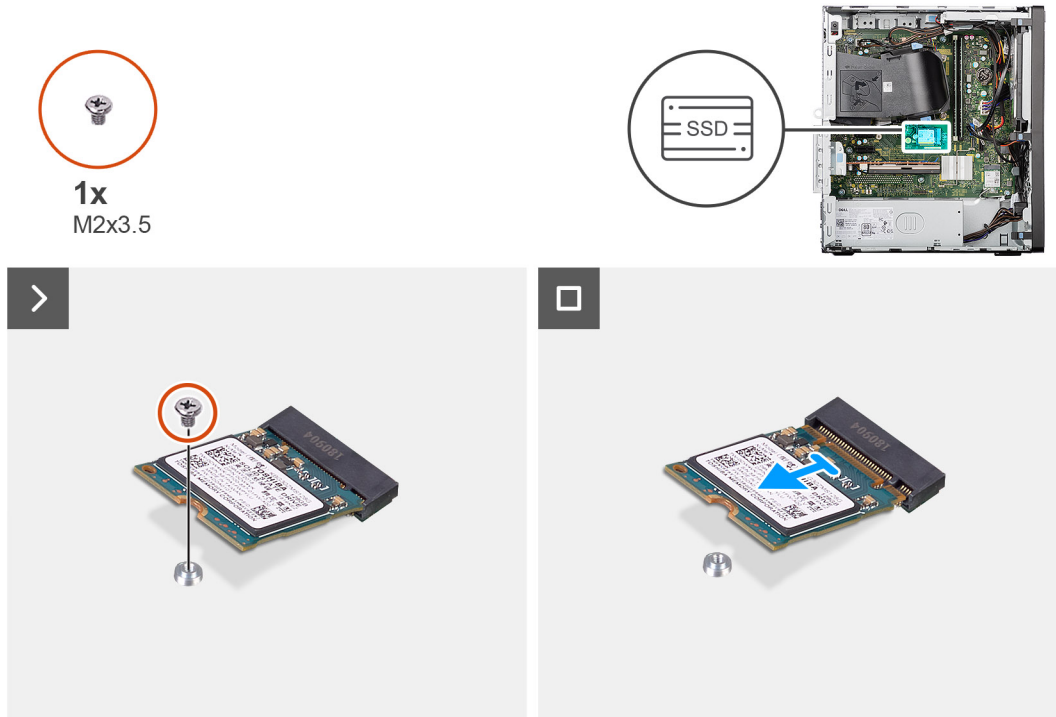
Figure 19. Removing the M.2 2230 solid-state drive
