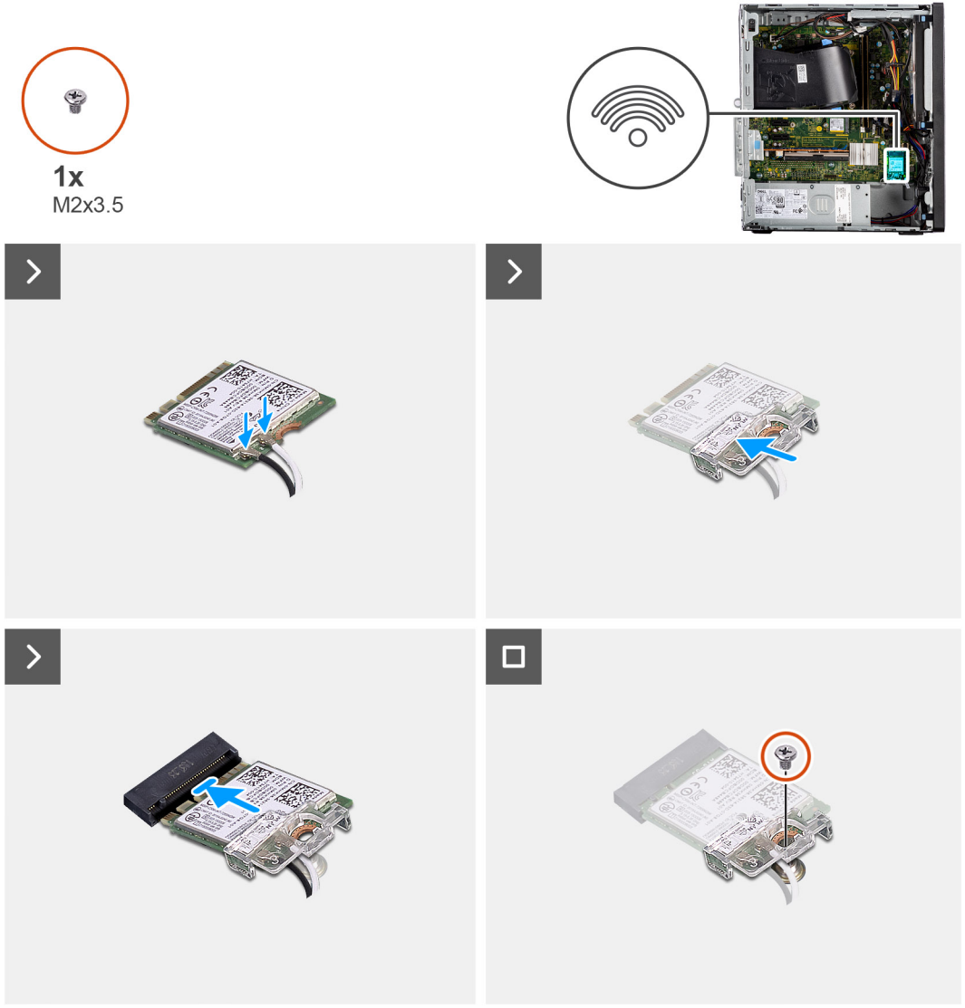
Figure 32. Installing the wireless card
