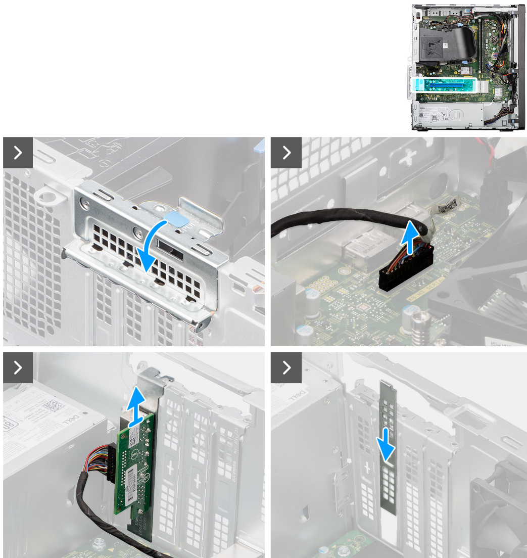
Figure 72. Removing the optional PS2 and serial module
