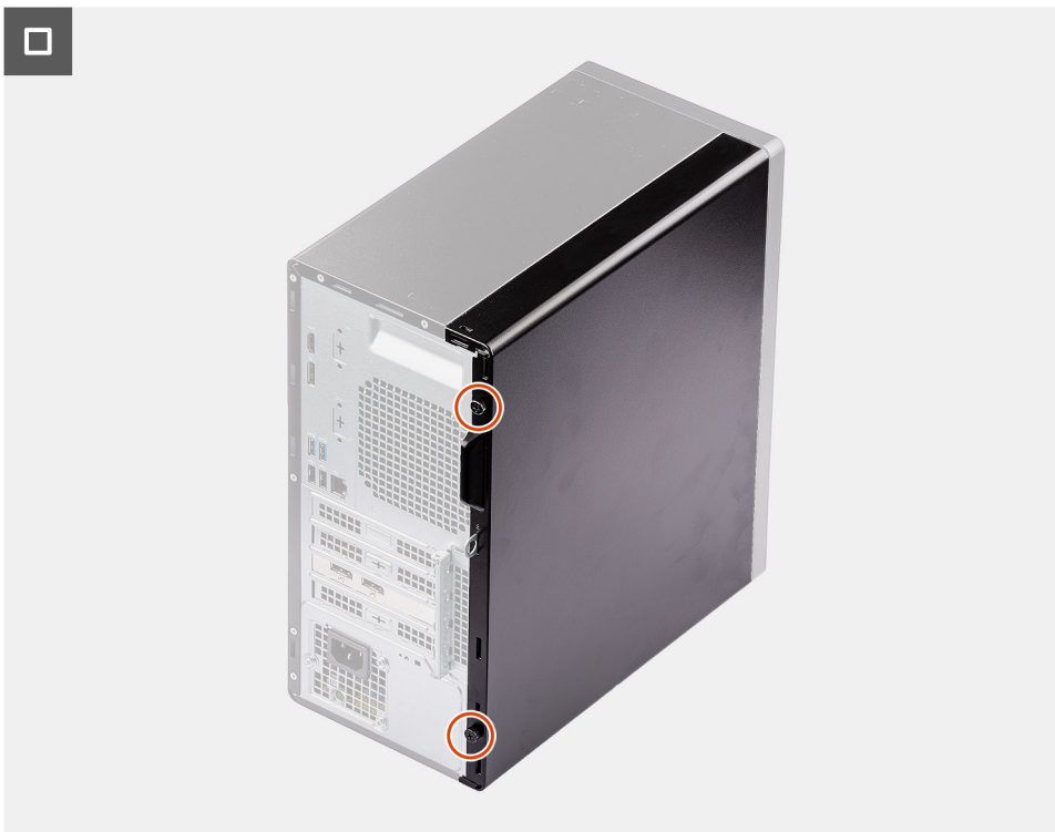
Figure 12. Installing the side cover
