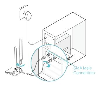
f. Replace the case panel, plug in the power cable and turn on your computer.
