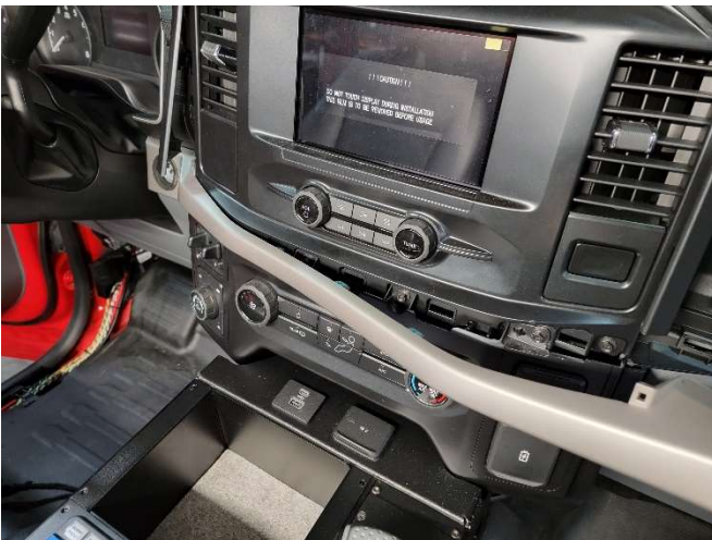
Temporarily reinstall the trim.
