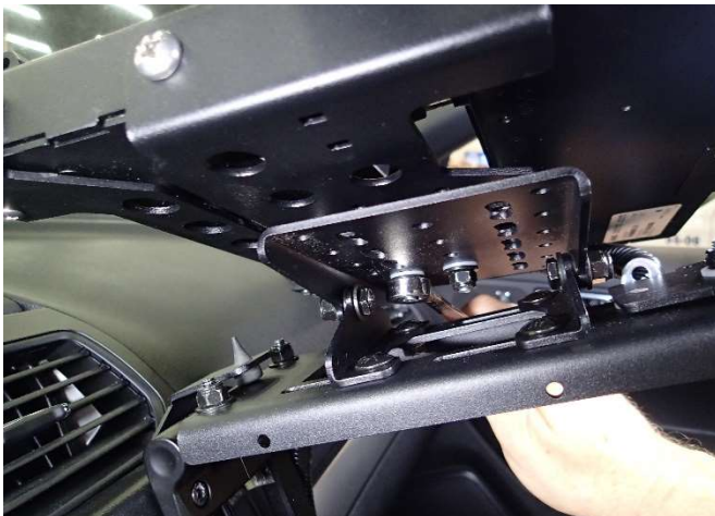
Determine desired position for your specific computer and attach to DMM swivel plate using 1/4" x 3/4" carriage bolts, PVC spacer, nylon washers, steel washers, and nylock nuts.
