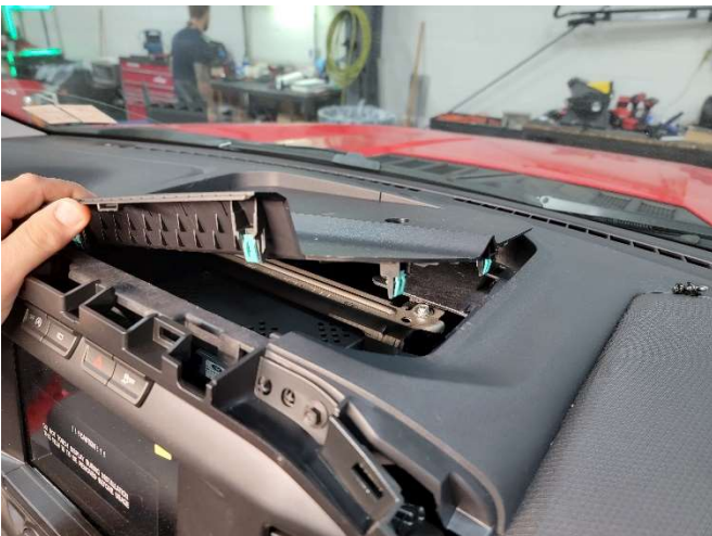
Lift off upper trim panel assembly. This panel will not be reused.
