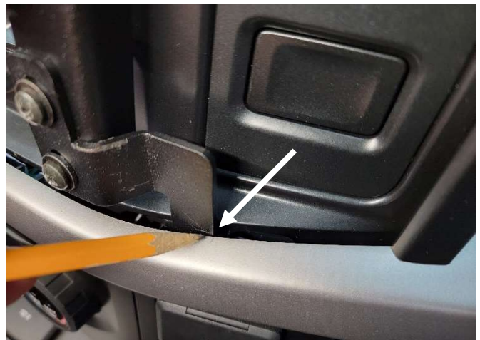
Mark location of trim coming into contact with lower mounting tab. Remove trim and cut away material as needed to clear bracket.
