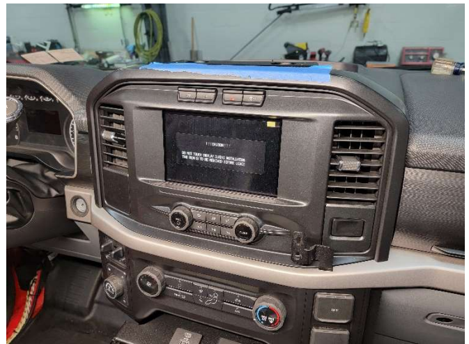
Reinstall previously removed trim around radio.
