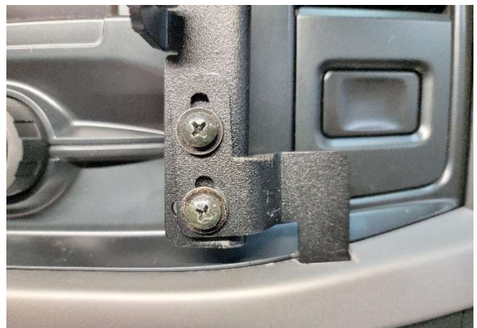
Attach frame support arm to lower mounting tab using (2) 10-32 x 1/2" machine screws, keps nuts and flat washers
