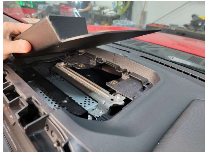
Place upper mounting tray onto dash.
