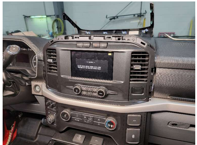
Remove trim around radio frame.
