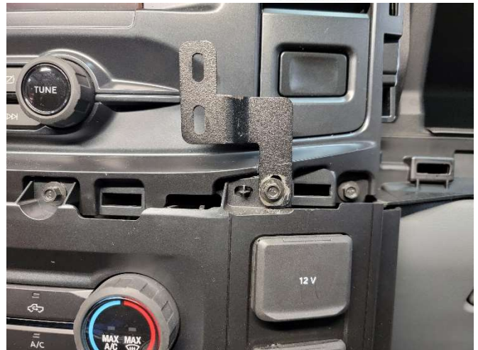
Install lower mounting tab using 7mm fastener.
