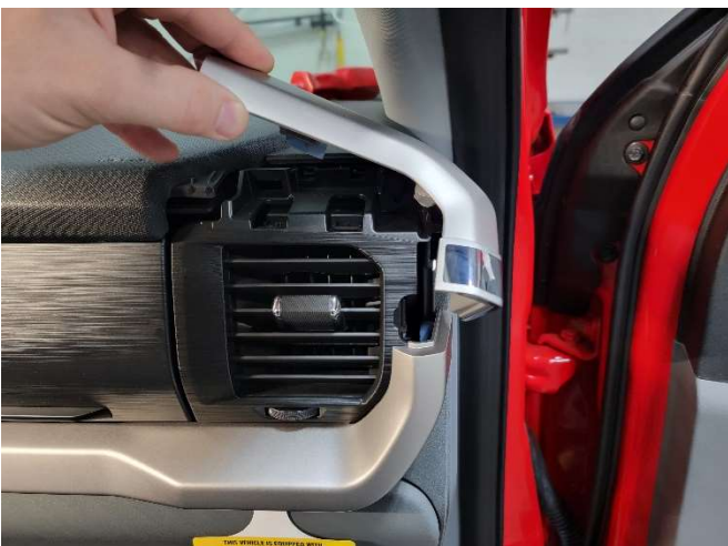
Unsnap trim around passenger vent assembly.
