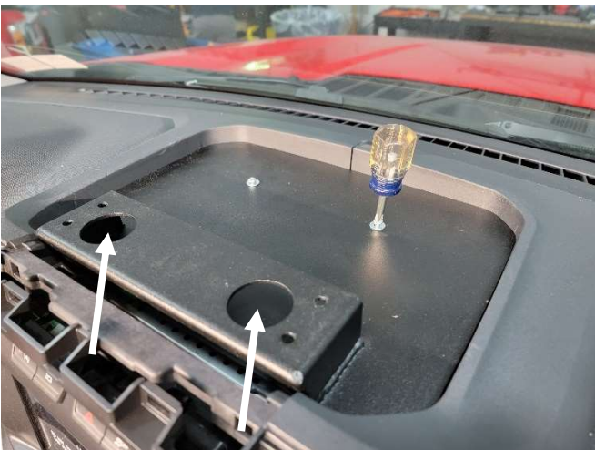
Attach using #8 x 1.5" pan head sheet metal screws in the front with flat washers and 10-32 x 3/4" machine screws in the rear with flat washers
