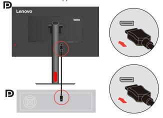
4. Connect one end of the DP cable to the DP input on the back of another monitor, and the other end to the DP output connector (for daisy chain) on the monitor.Note 1: Monitors sold in NA include an DP cable.Note 2: For other regions Lenovo recommends that customers who require to use the Display Port input on their monitor purchase the "Lenovo Display Port to Display Port cable 0A36537". For more information, go to one of the following: www.lenovo.com/support/monitor accessories.
