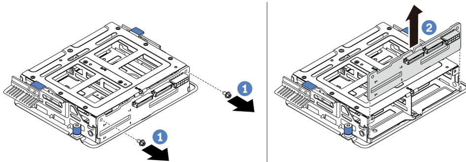
Figure 137. Internal backplane removal
