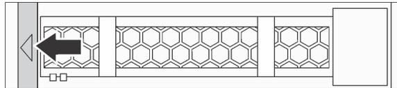
Figure 85. Opening the drive tray handle
