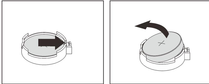
Figure 122. CMOS battery removal
