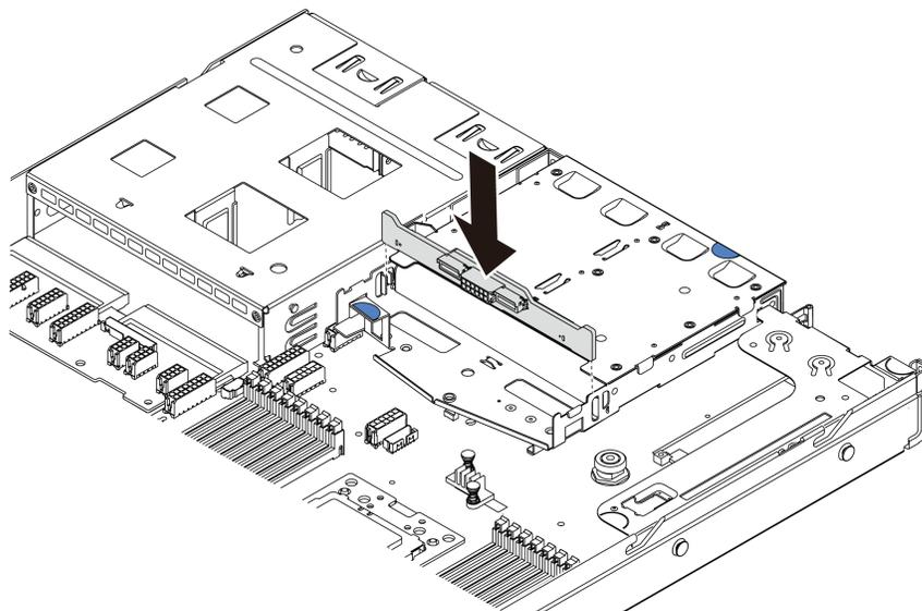
Figure 118. Rear backplane installation
