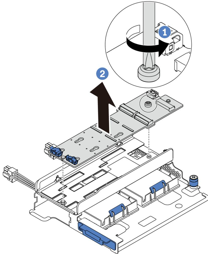
Figure 144. M.2 adapter removal
