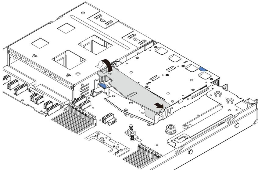
Figure 121. Air baffle installation
