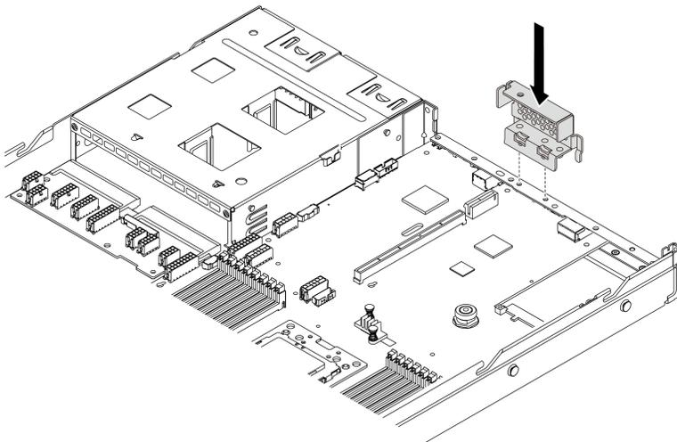
Figure 101. Rear wall bracket installation
