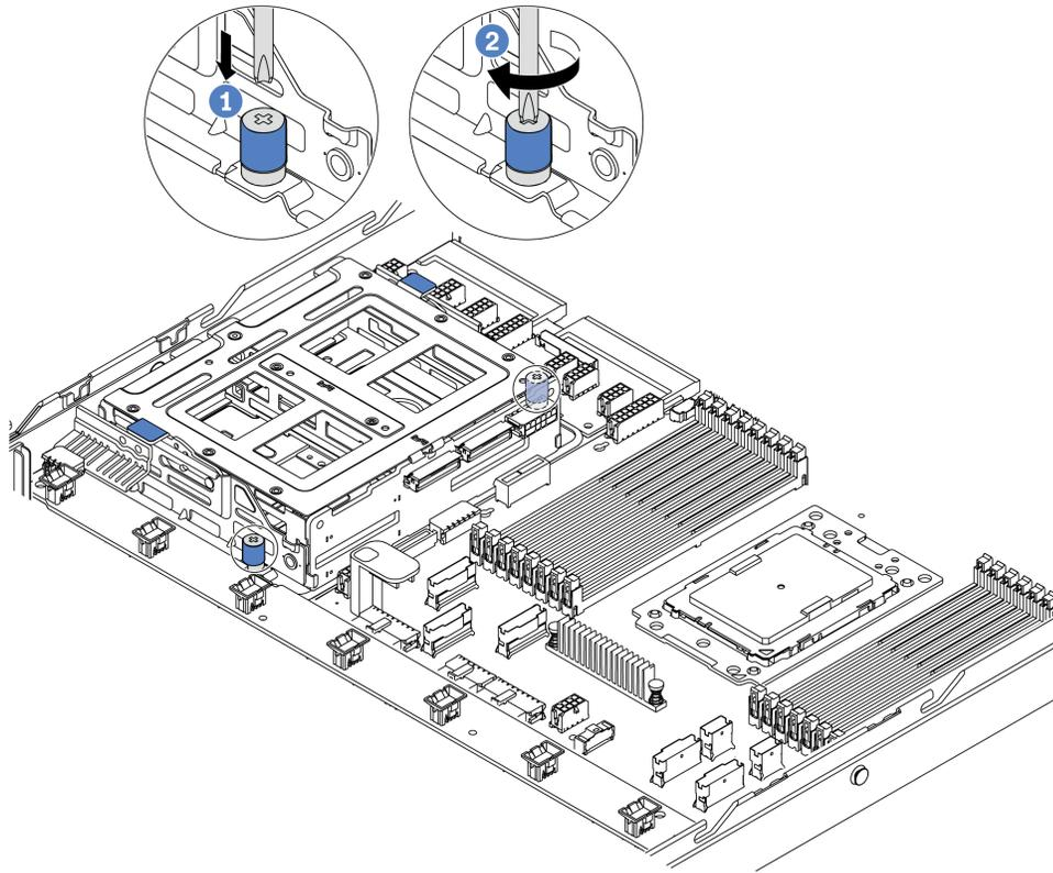
Figure 140. Middle drive cage installation-2
