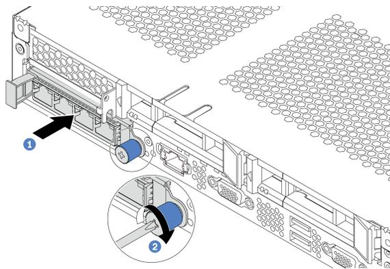
Figure 91. OCP 3.0 Ethernet adapter installation
