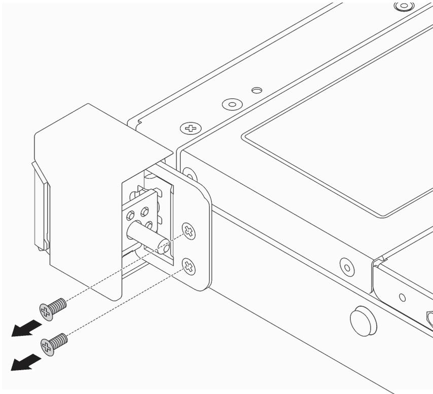
Figure 71. Rack latch screws removal
