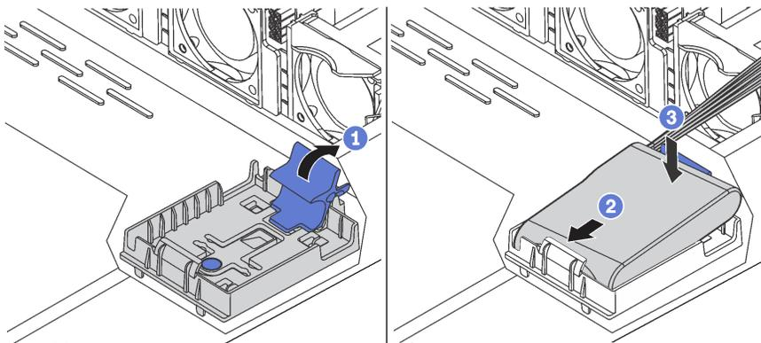
Figure 157. Installation of the RAID super capacitor module on the chassis
