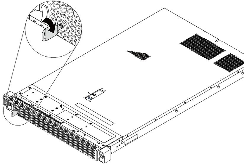
Figure 76. Security bezel unlock
