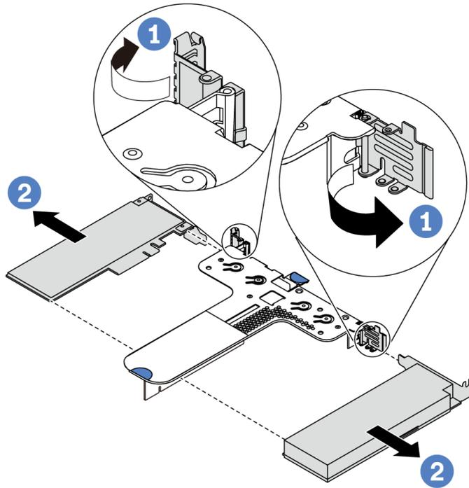
Figure 103. Riser 2 assembly (LP+LP) removal
