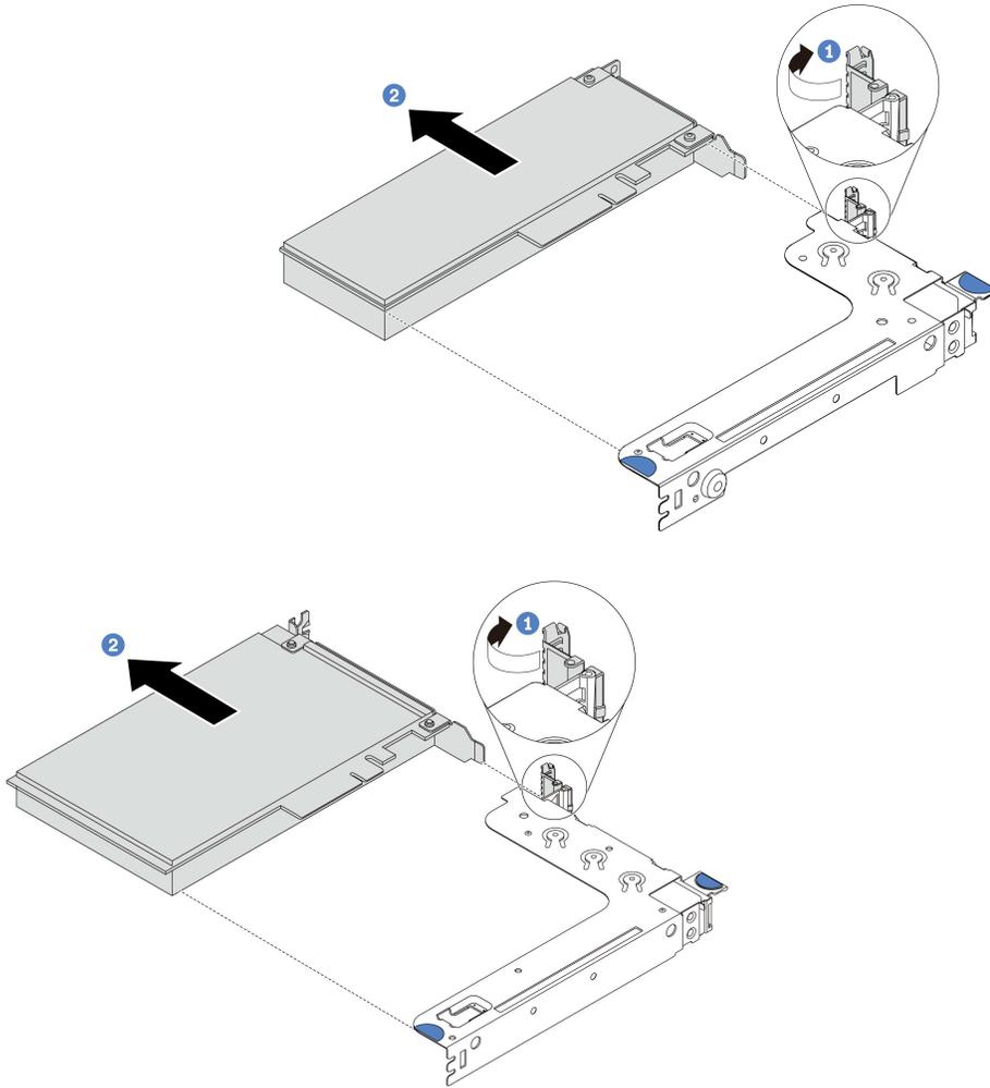
Figure 102. Riser 1 assembly (LP/FHFL) removal
