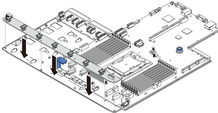
Figure 175. Fan board installation
