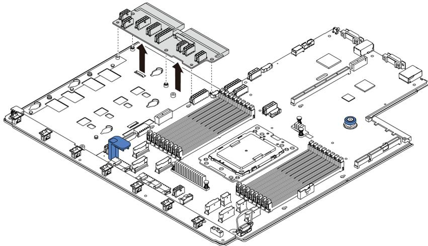
Figure 176. PIB board removal
