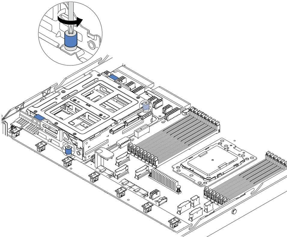
Figure 135. Middle drive cage removal-1
