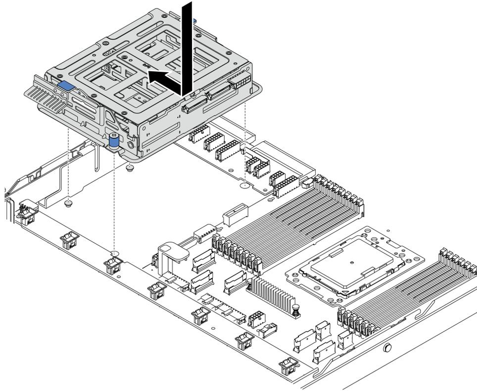
*Figure 139. Middle drive cage installation-1*
