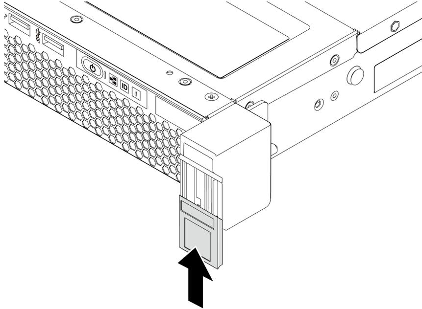
Figure 75. ID label plate installation
