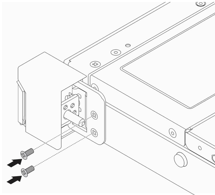
*Figure 74. Rack latch screws installation*
