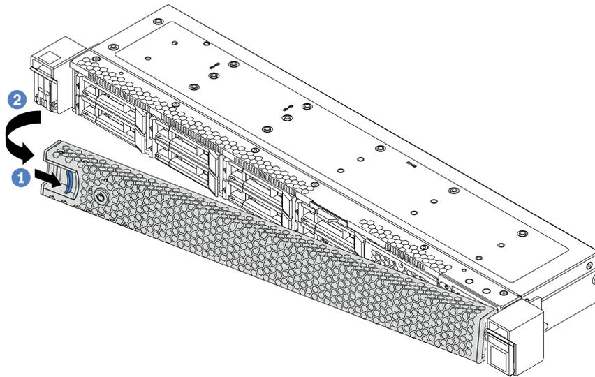
Figure 77. Security bezel removal
