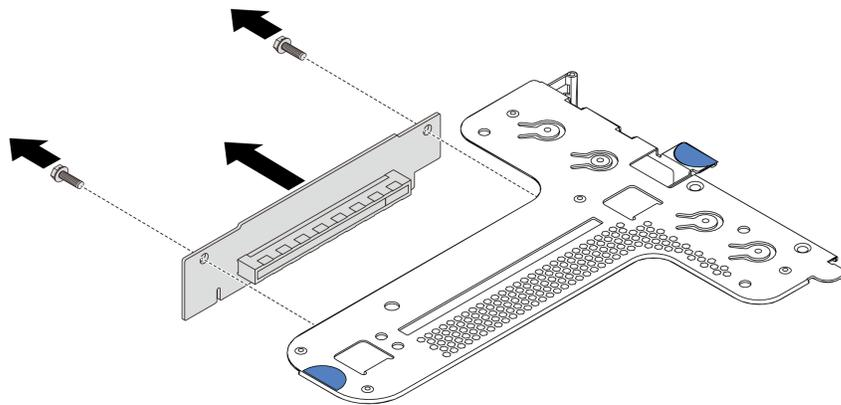
Figure 98. Riser card removal
