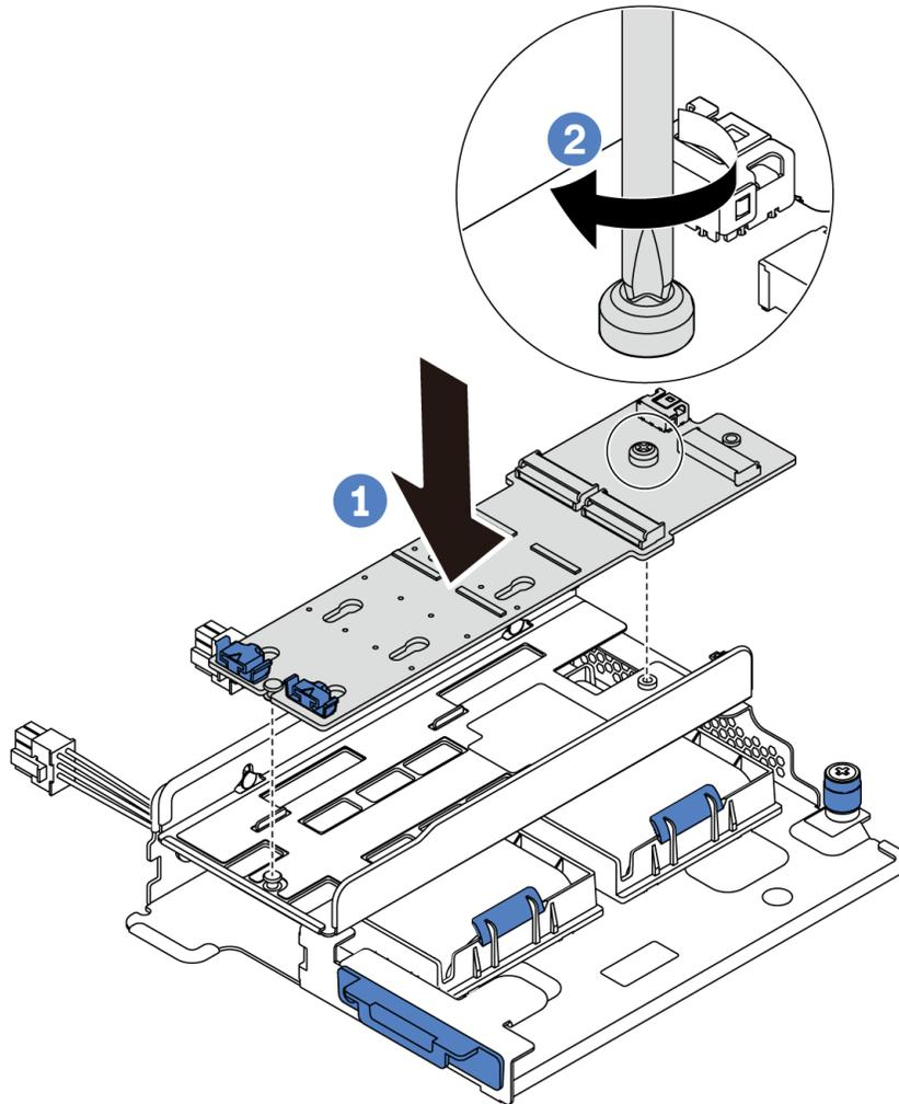
Figure 149. M.2 adapter installation
