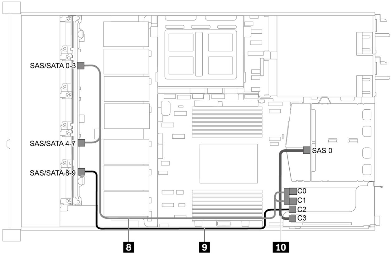
Figure 52. Cable routing for server model with ten 2.5-inch SAS/SATA/NVMe drives, rear SAS/SATA drive assembly, middle NVMe drive assembly and one 16i RAID/HBA adapter-2
