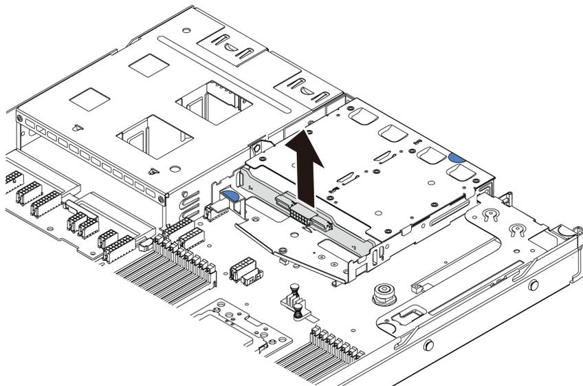
Figure 117. Rear backplane removal
