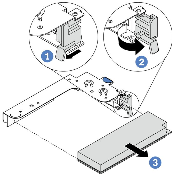
Figure 104. Internal riser assembly (LP) removal
