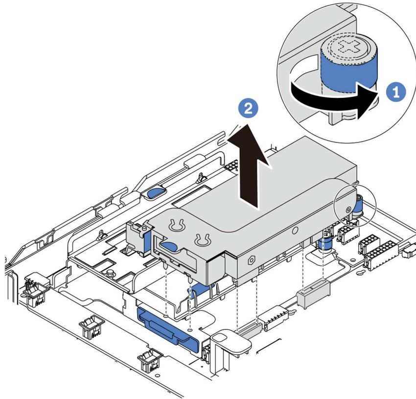
Figure 92. Internal riser assembly removal
