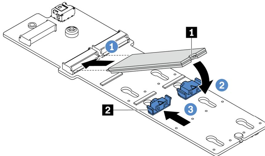
Figure 150. M.2 drive installation
