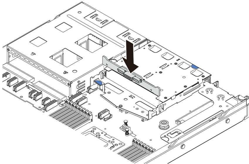
Figure 128. Rear backplane installation
