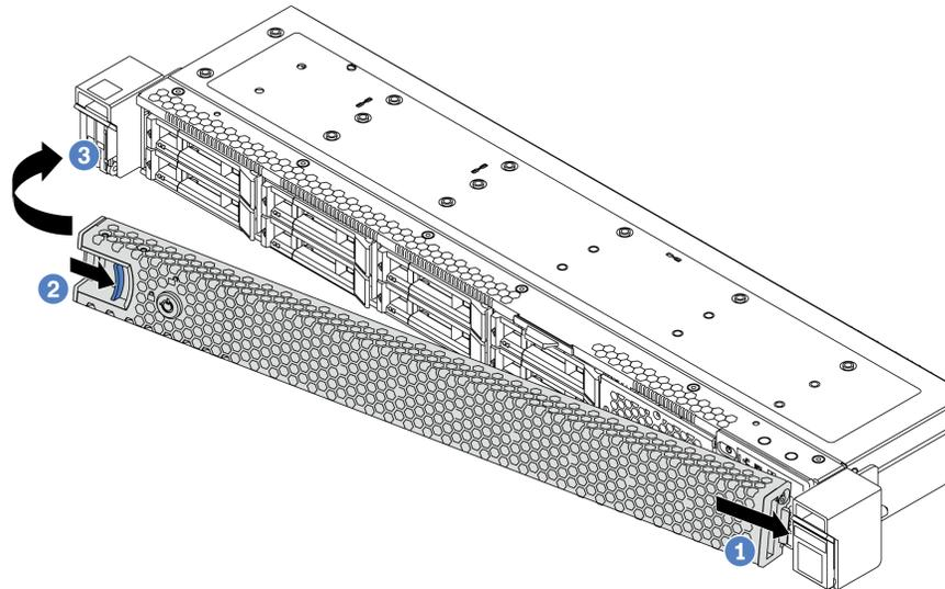
Figure 79. Security bezel installation
