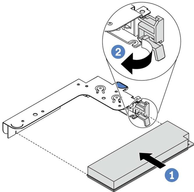
Figure 107. Internal riser assembly (LP) installation
