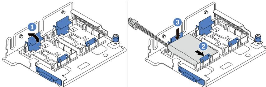
Figure 152. Super capacitor module installation
