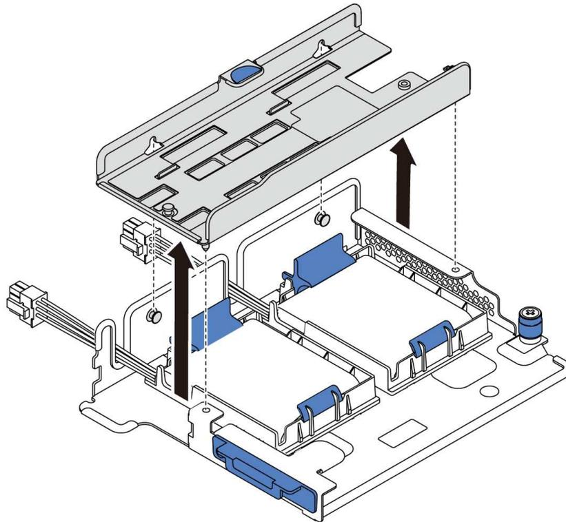
Figure 145. M.2 adapter bracket removal
