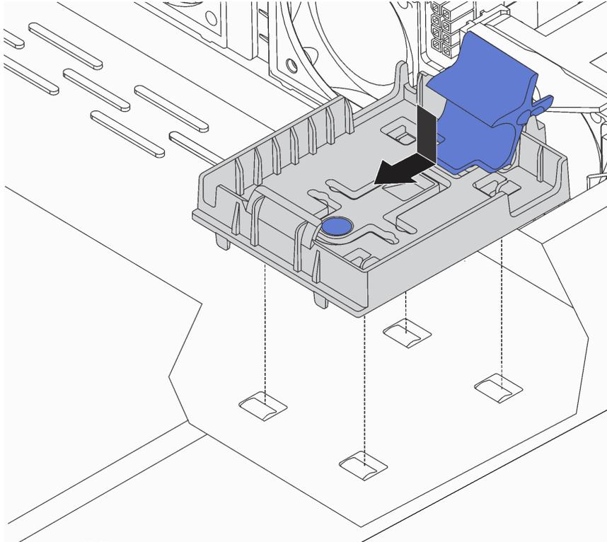
Figure 156. RAID super capacitor module holder installation
