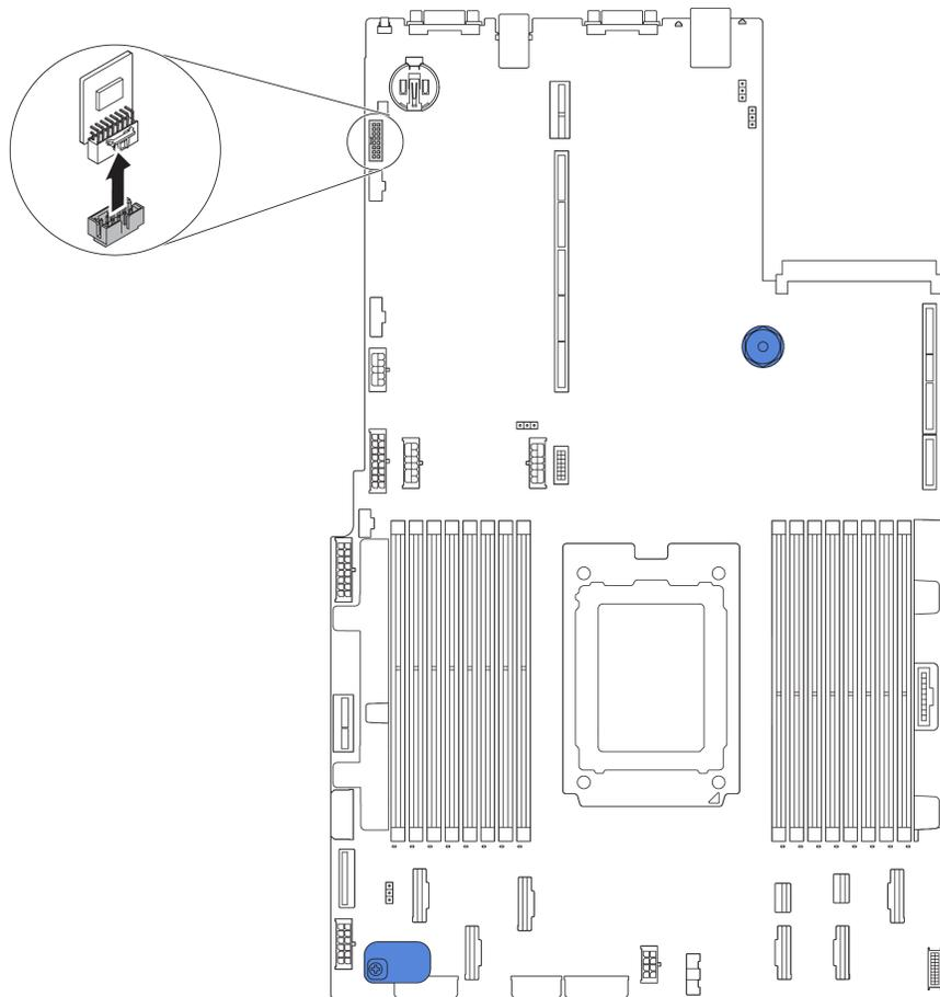
Figure 124. TPM adapter removal
