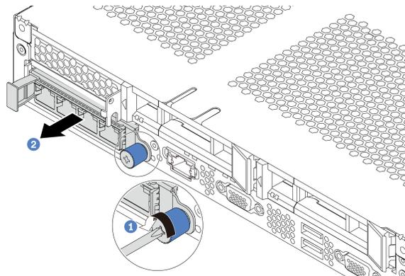
Figure 89. OCP 3.0 Ethernet adapter removal
