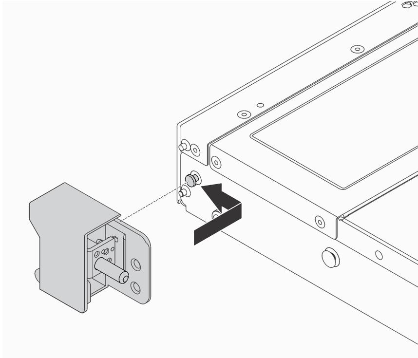
*Figure 73. Rack latch installation*
