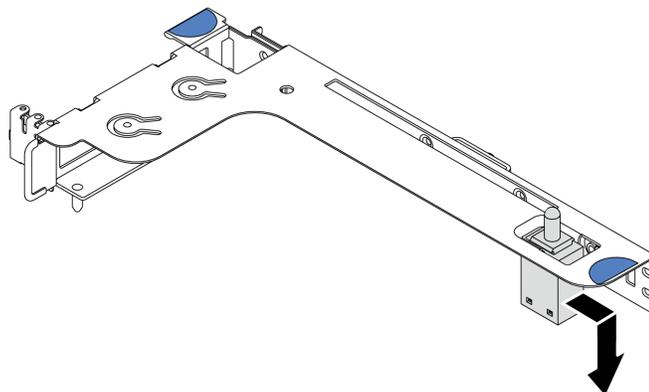
Figure 108. Intrusion switch removal
