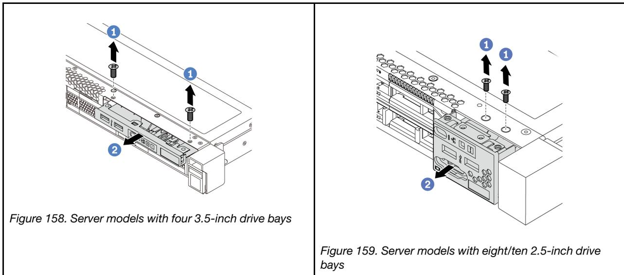
Step 1. Remove the screws that secure the front I/O assembly.
