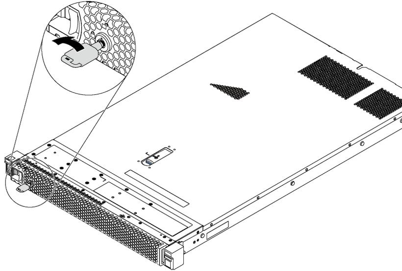
Figure 80. Security bezel lockup
