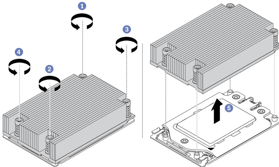
Figure 169. Removing a heat sink
