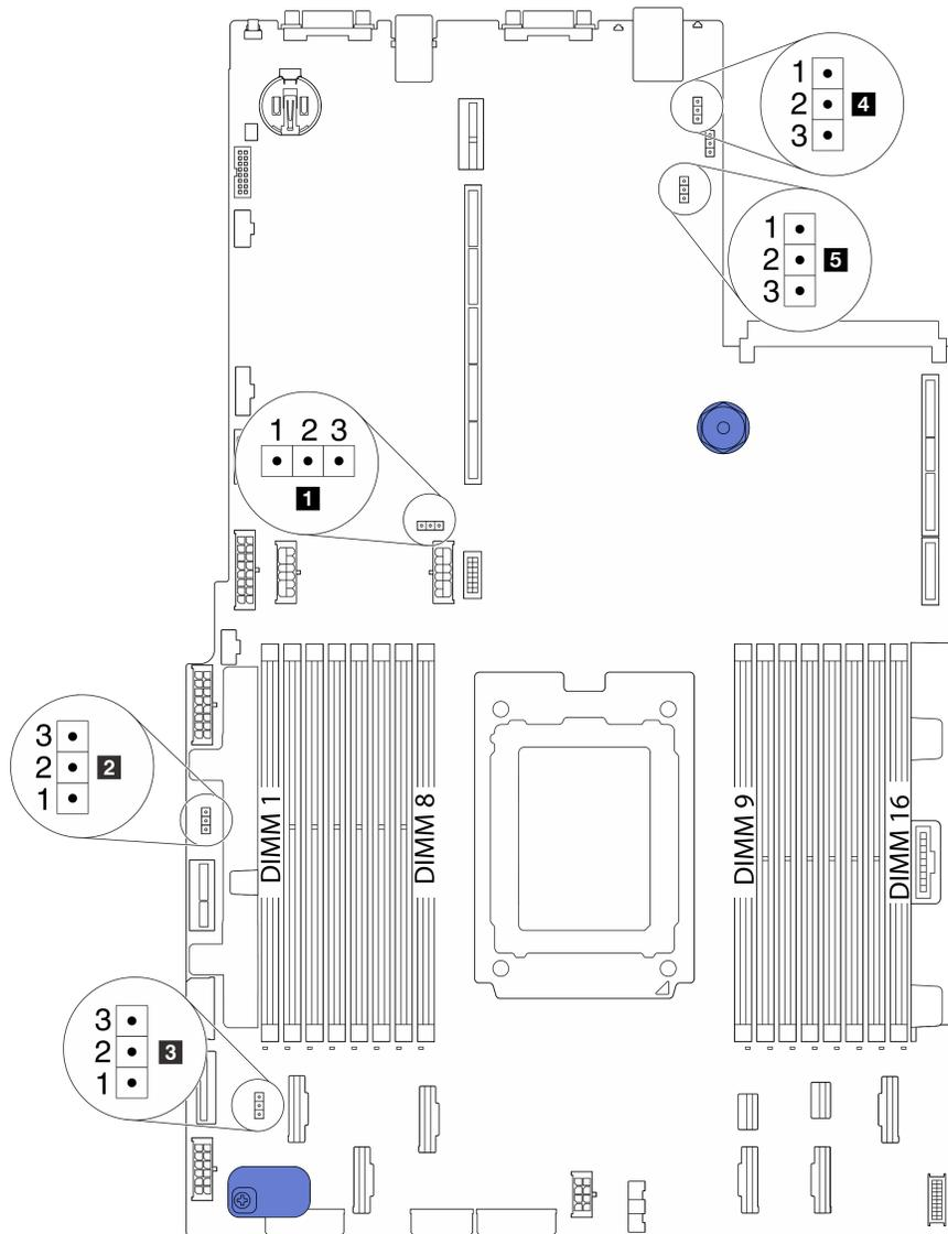
Figure 17. System board jumpers
