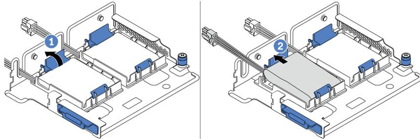
Figure 151. Super capacitor module removal
