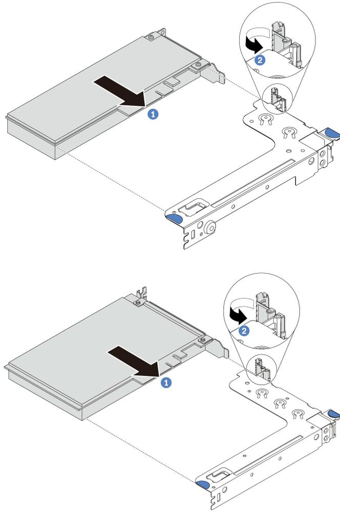
Figure 105. Riser 1 assembly (LP/FHFL) installation
