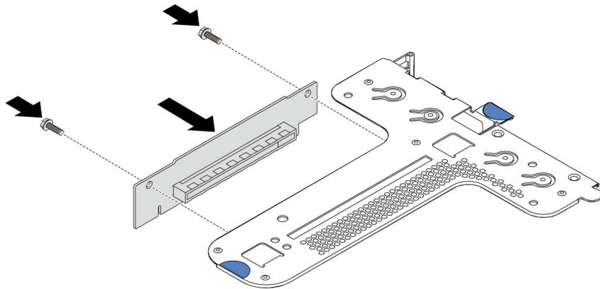
Figure 99. Riser card installation
