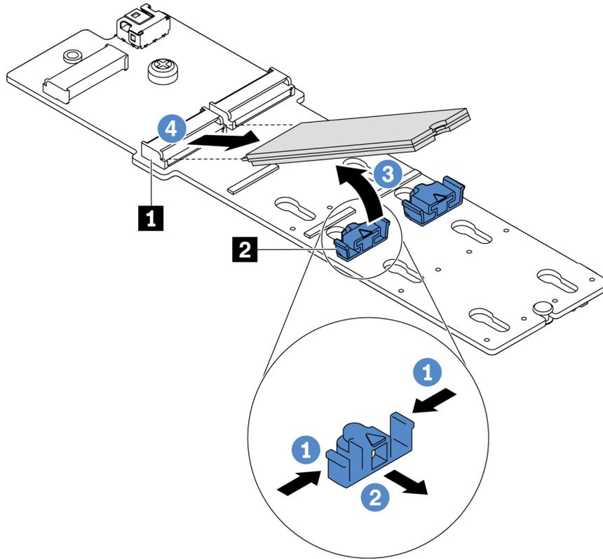
Figure 143. M.2 drive removal
