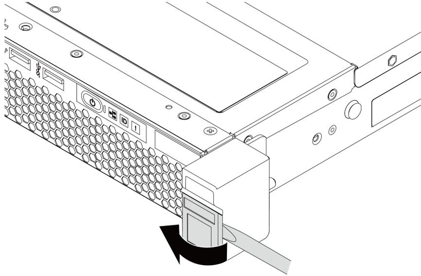
Figure 70. ID label plate removal
