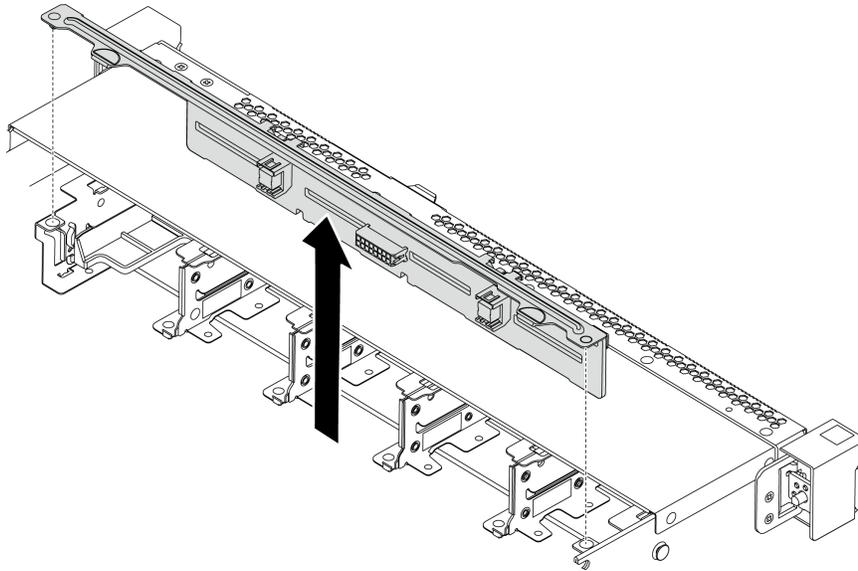
Figure 112. Removal of backplane for eight 2.5-inch hot-swap drives
