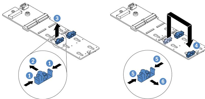
Figure 146. M.2 retainer adjustment
