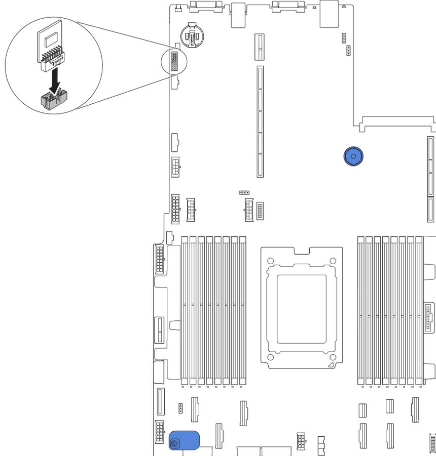
Figure 125. TPM adapter installation
