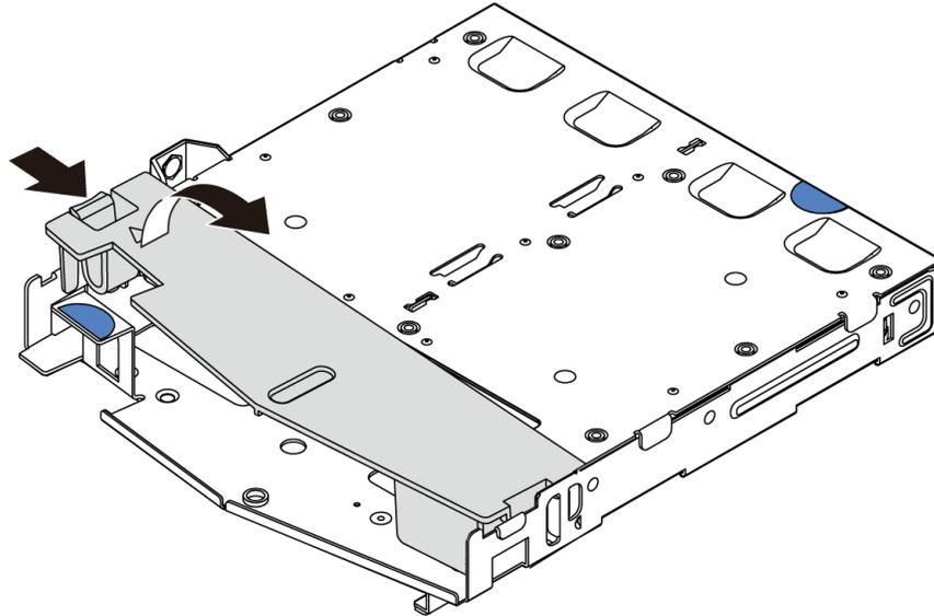
Figure 127. Air baffle removal
