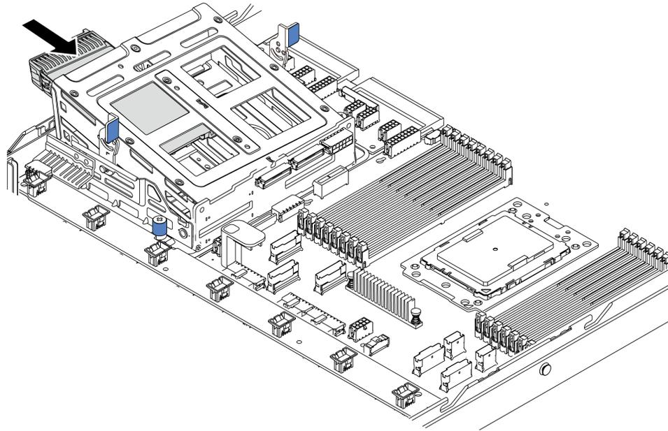
Figure 142. Internal hot-swap drive installation-2
