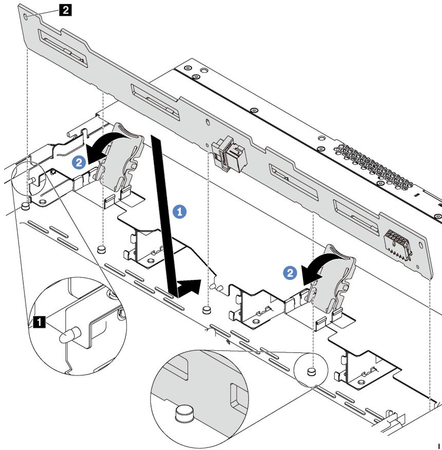
Figure 111. Installation of backplane for four 3.5-inch hot-swap drives
