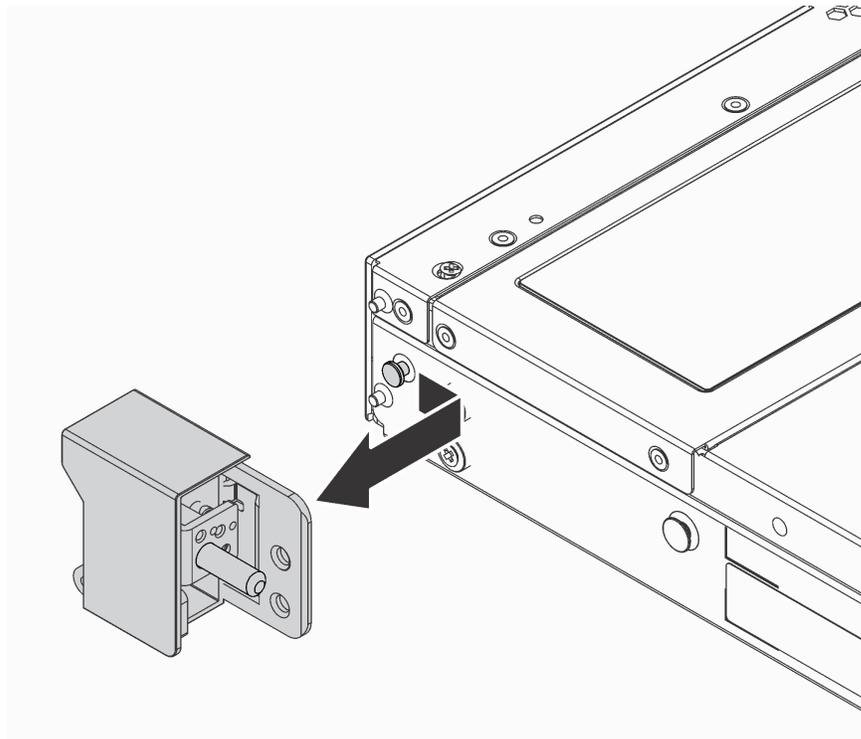
Figure 72. Rack latch removal
