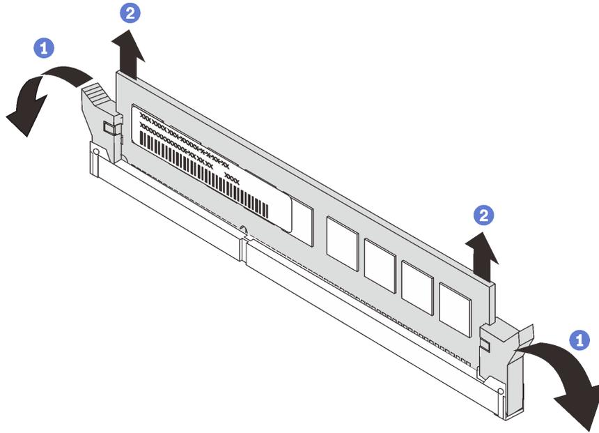
Figure 83. Memory module removal
