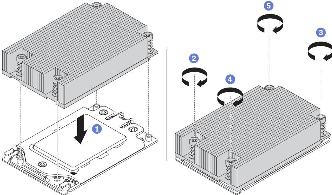
Figure 173. Installing a heat sink
