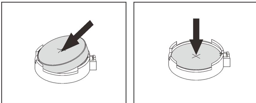
Figure 123. CMOS battery installation
