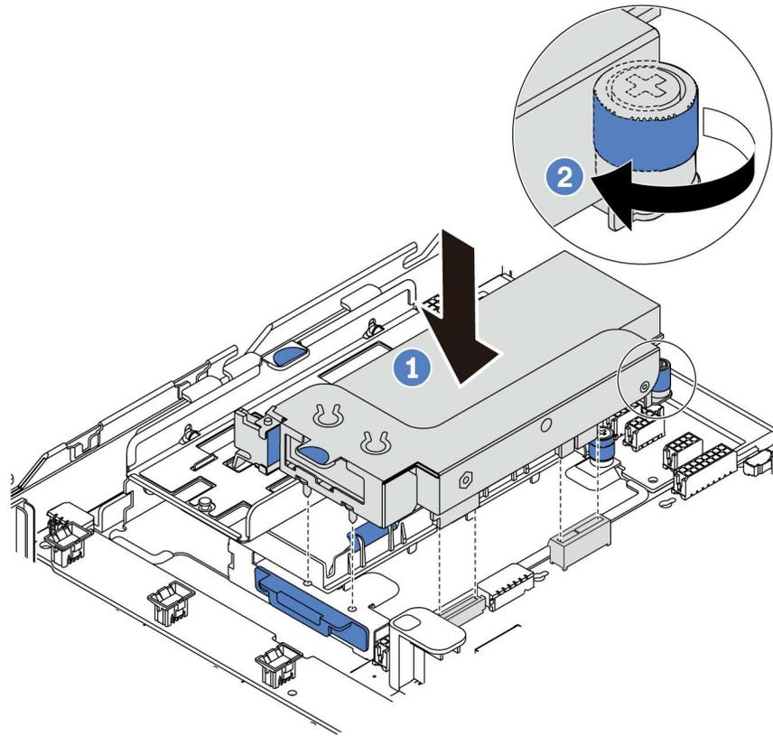
Figure 93. Internal riser assembly installation
