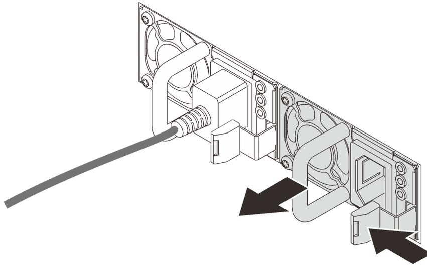
Figure 164. Hot-swap power supply removal
