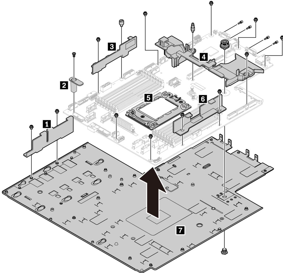
Figure 182. Disassembling the system board
