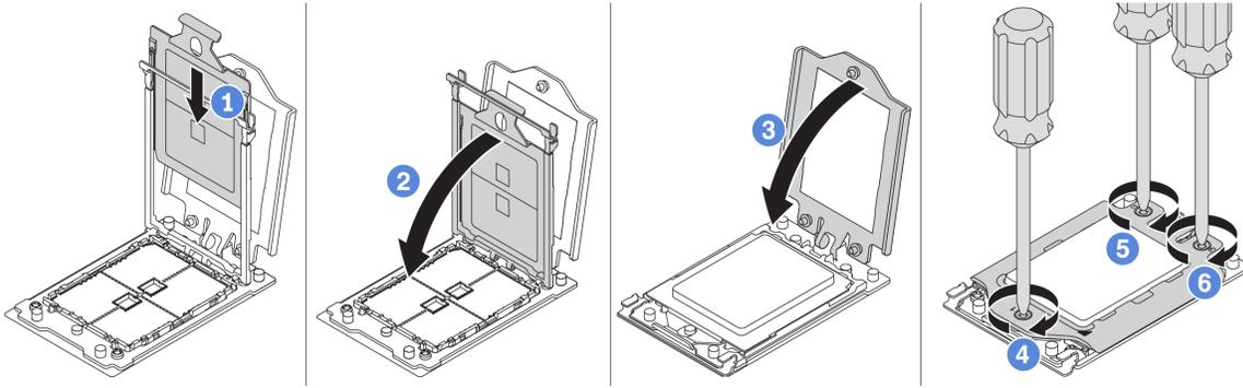
Figure 171. Installing a processor
