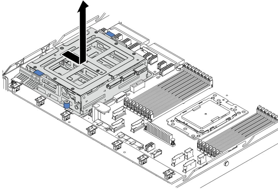
Figure 136. Middle drive cage removal-2
