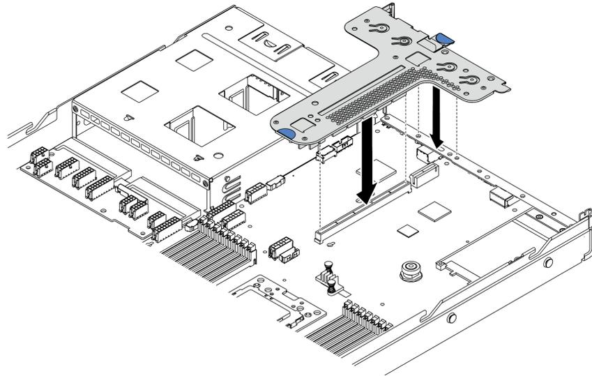
Figure 100. Riser assembly installation
