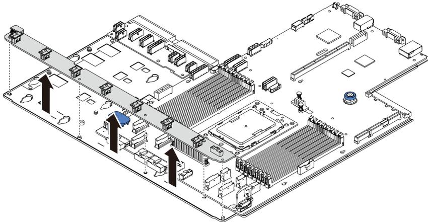
Figure 174. Fan board removal
