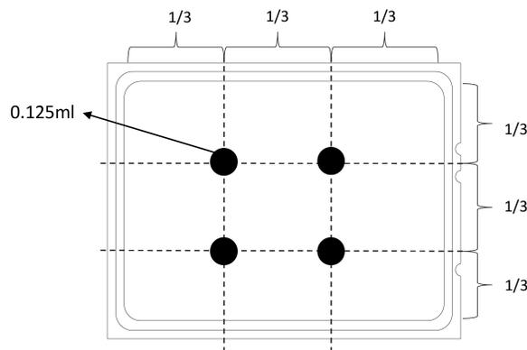
Figure 172. Applying thermal grease
