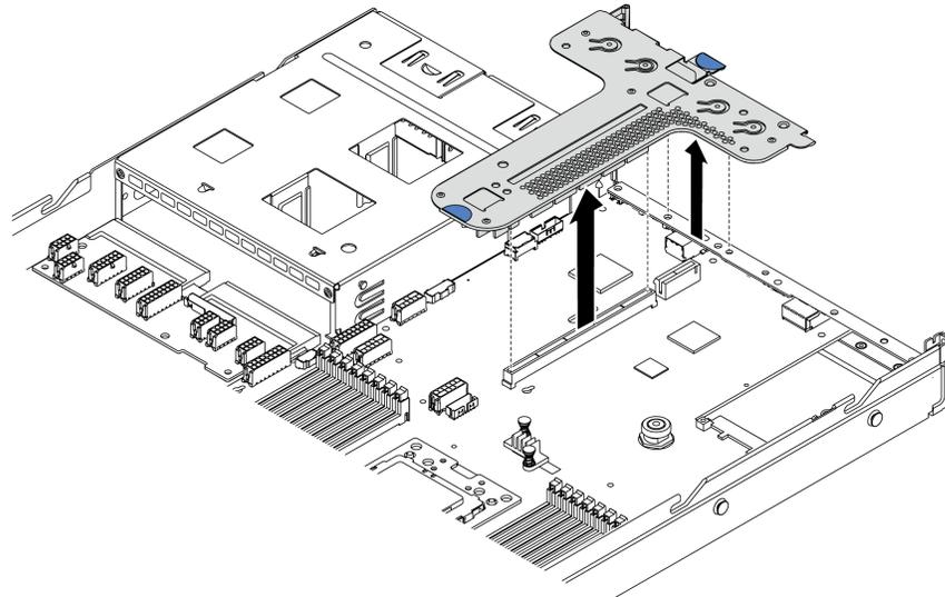
Figure 97. Riser assembly removal
