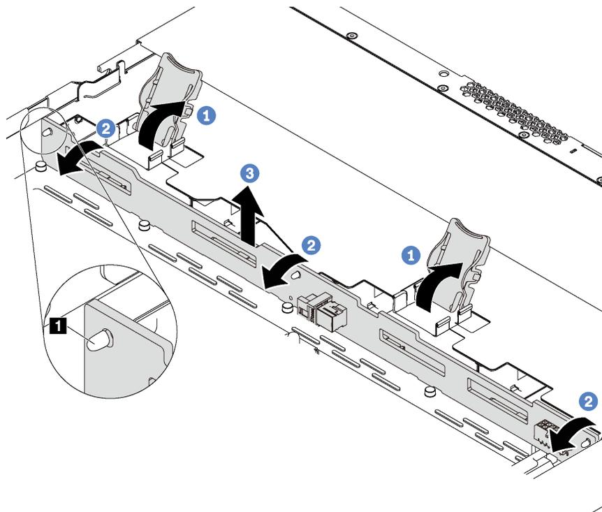
Figure 110. Removal of backplane for four 3.5-inch hot-swap drives
