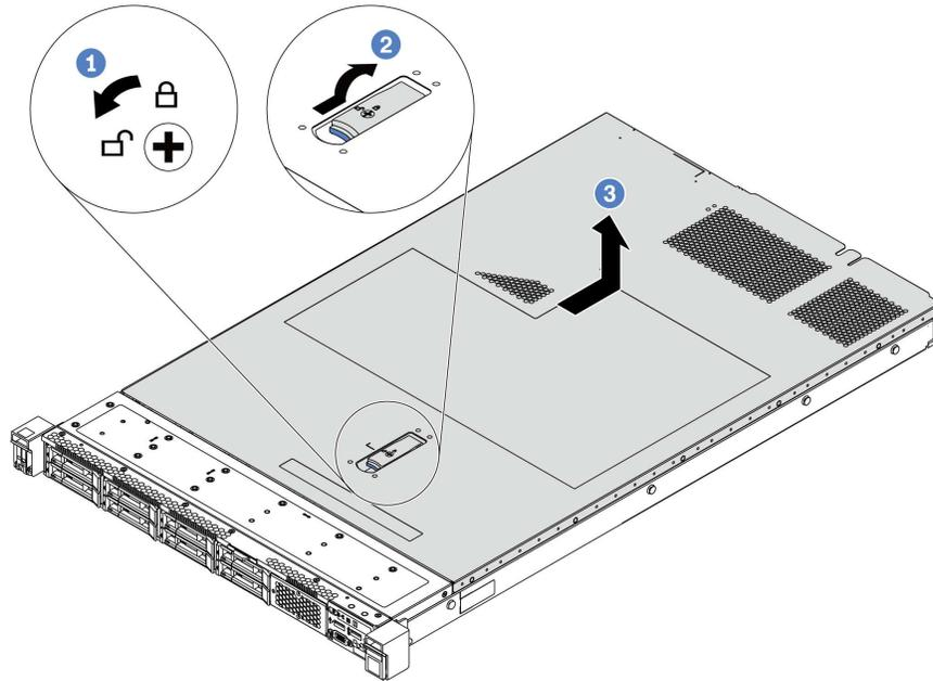
Figure 66. Top cover removal
