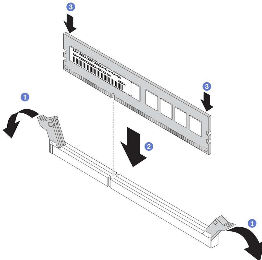
Figure 84. Memory module installation
