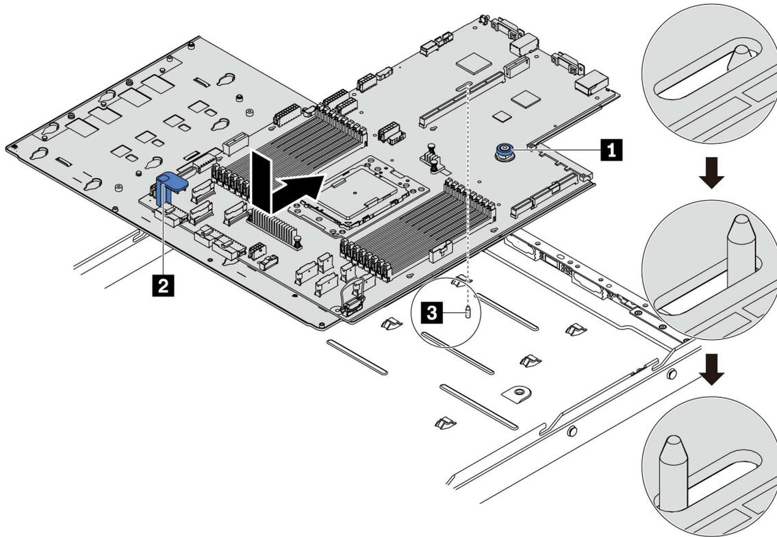
Figure 179. System board installation
