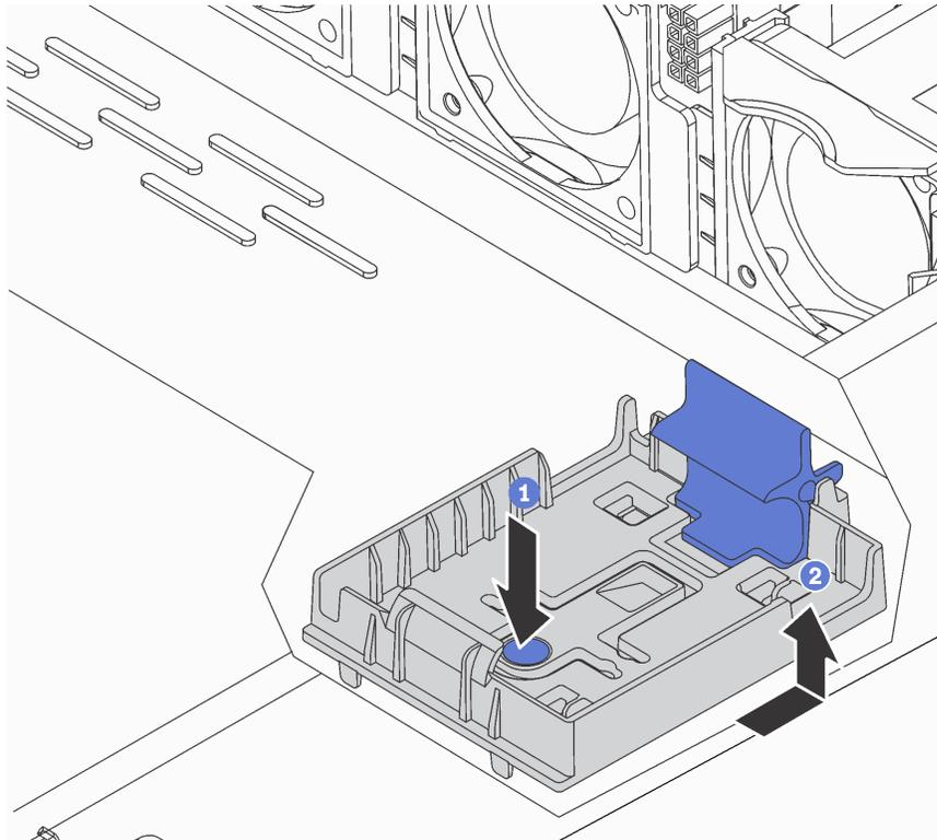
Figure 154. RAID super capacitor module holder removal
