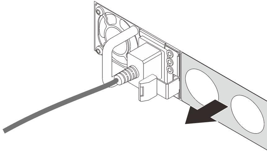
Figure 167. Hot-swap power supply filler removal
