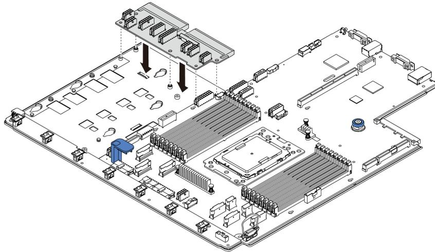
Figure 177. PIB board installation
