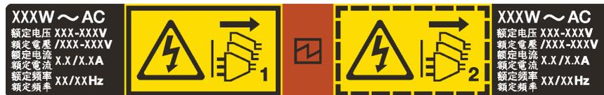
Figure 165. Hot-swap power supply label on the cover
