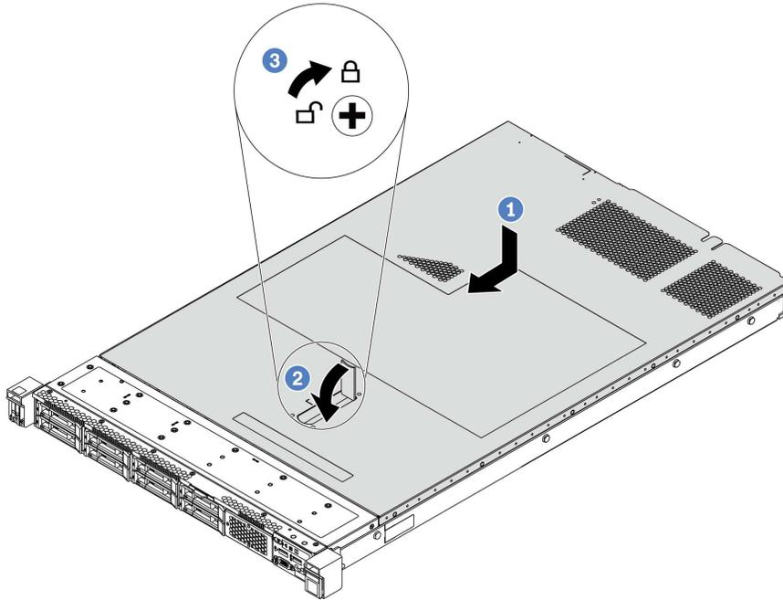
Figure 67. Top cover installation
