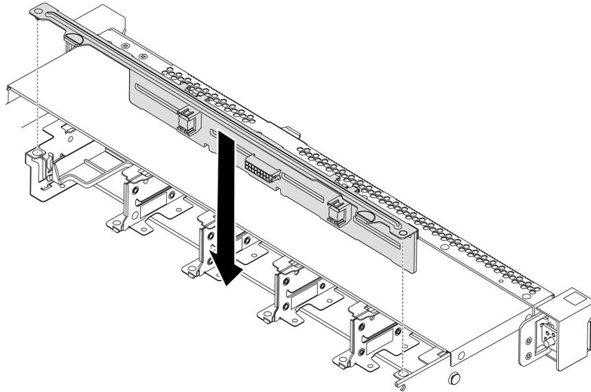
Figure 113. Installation of backplane for eight 2.5-inch hot-swap drives
