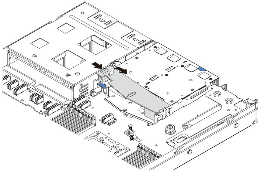
Figure 116. Air baffle removal
