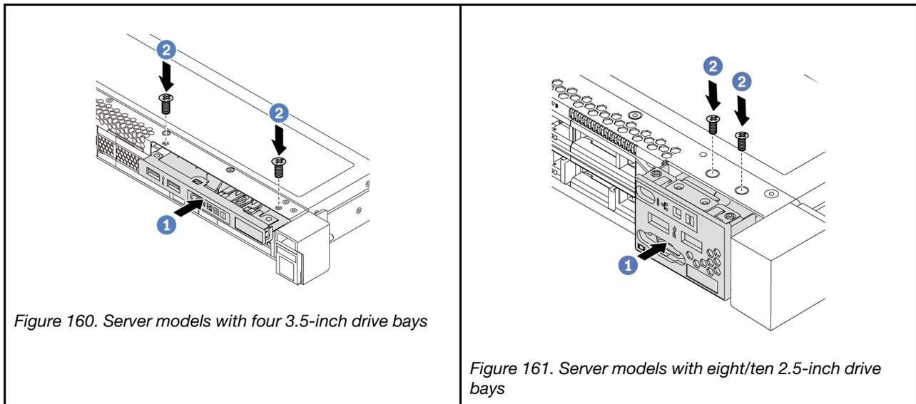
Step 1. Insert the front I/O assembly into the assembly bay.
