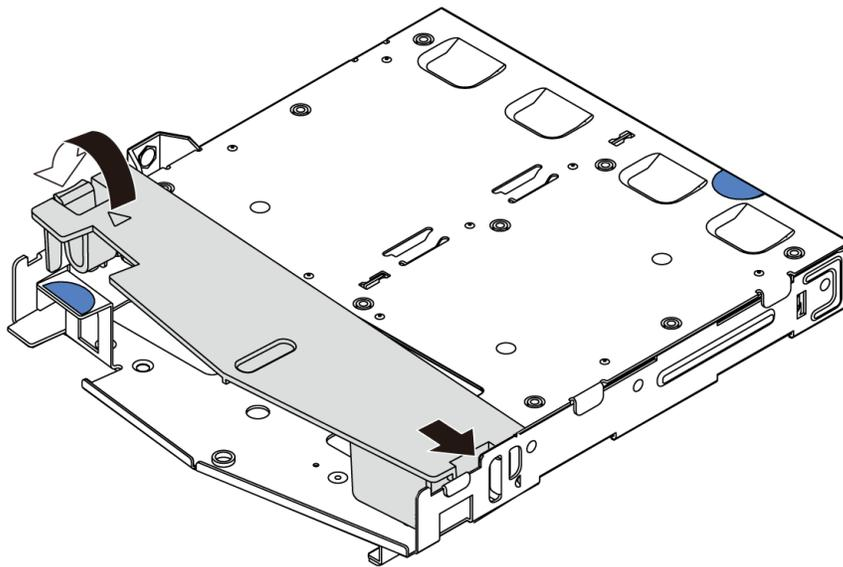
Figure 131. Air baffle installation
