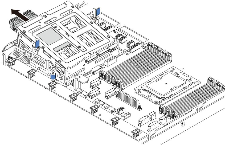
Figure 134. Internal drive removal-2
