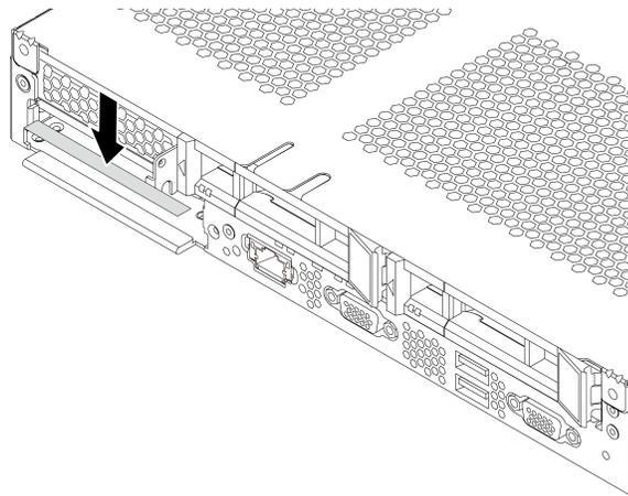
*Figure 90. OCP 3.0 Ethernet adapter label installation*
