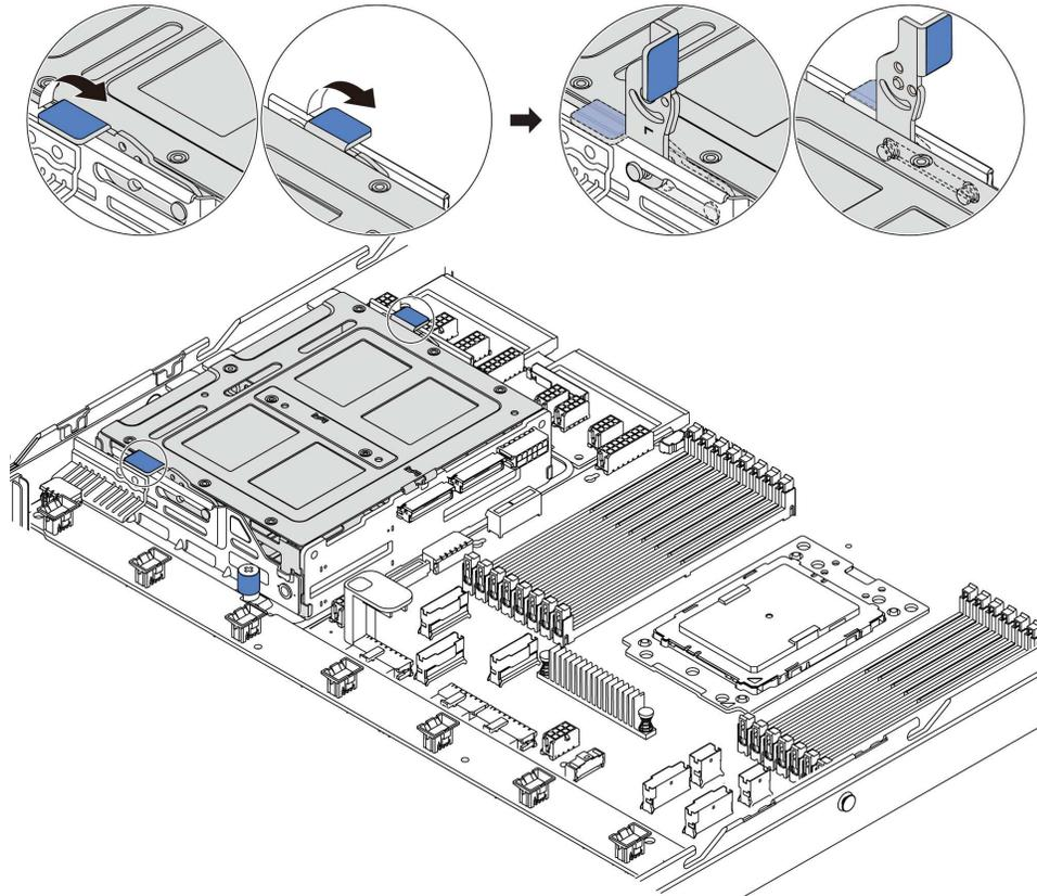
Figure 133. Internal drive removal-1
