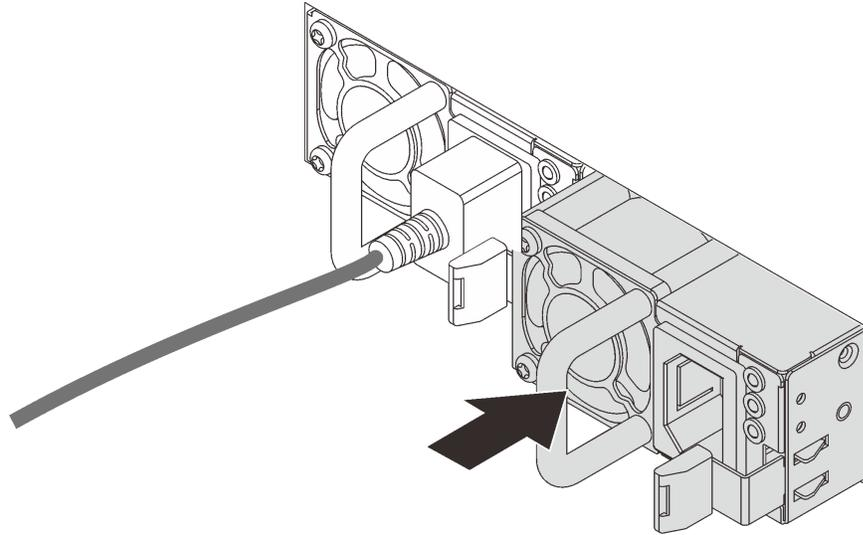
Figure 168. Hot-swap power supply installation
