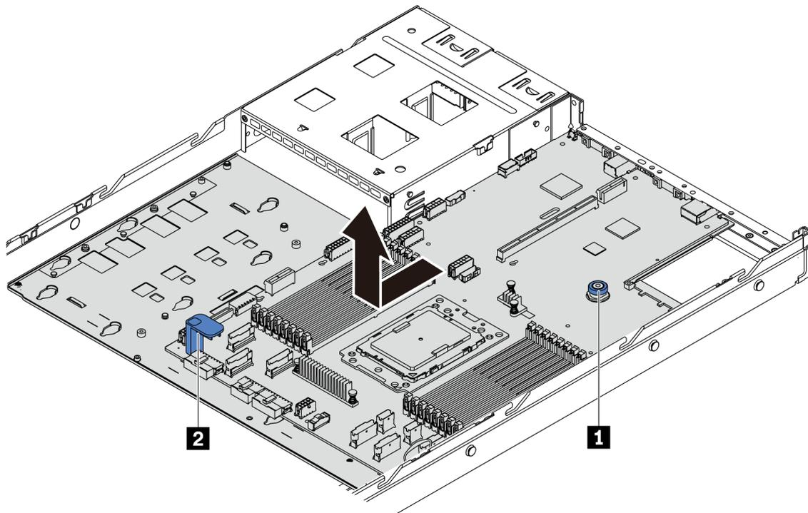
Figure 178. System board removal
