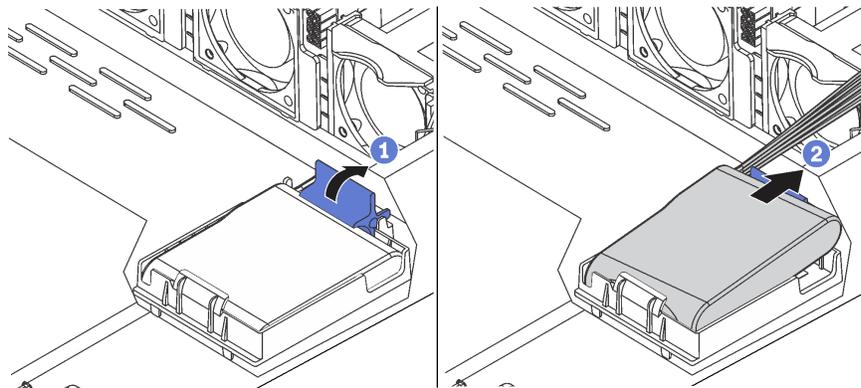
Figure 153. Removal of the RAID super capacitor module on the chassis
