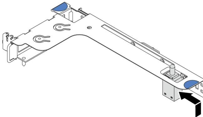
Figure 109. Intrusion switch installation
