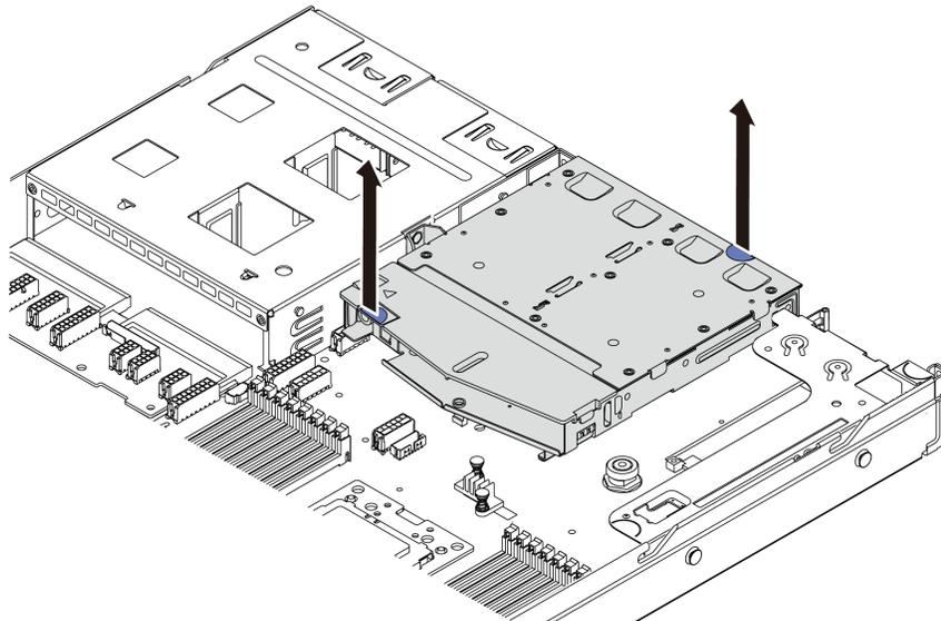
Figure 126. Rear hot-swap drive cage removal
