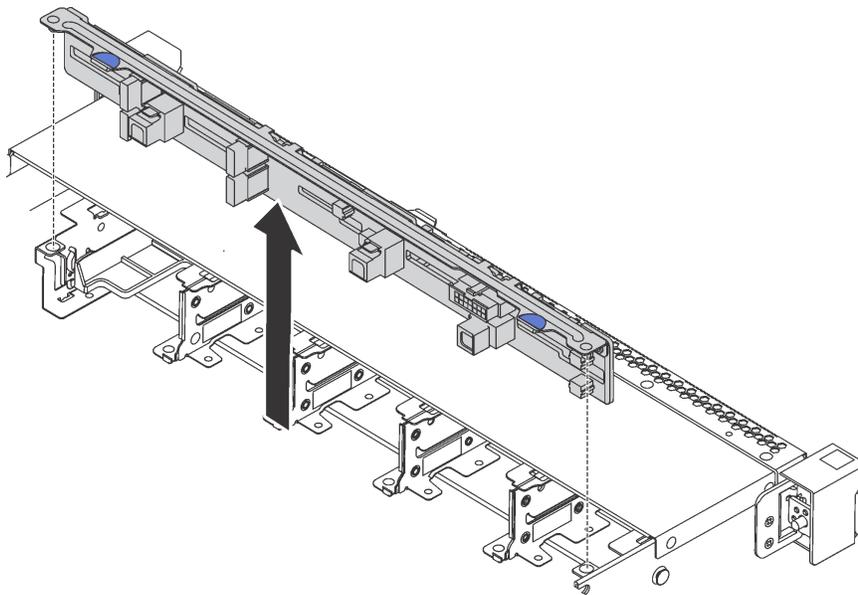
Figure 114. Removal of backplane for ten 2.5-inch hot-swap drives
