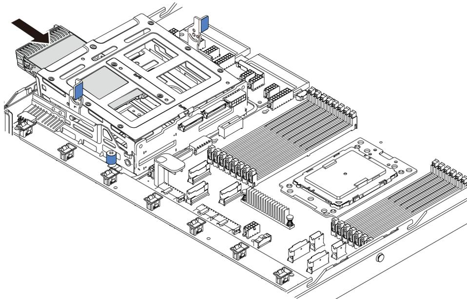
Figure 141. Internal hot-swap drive installation-1
