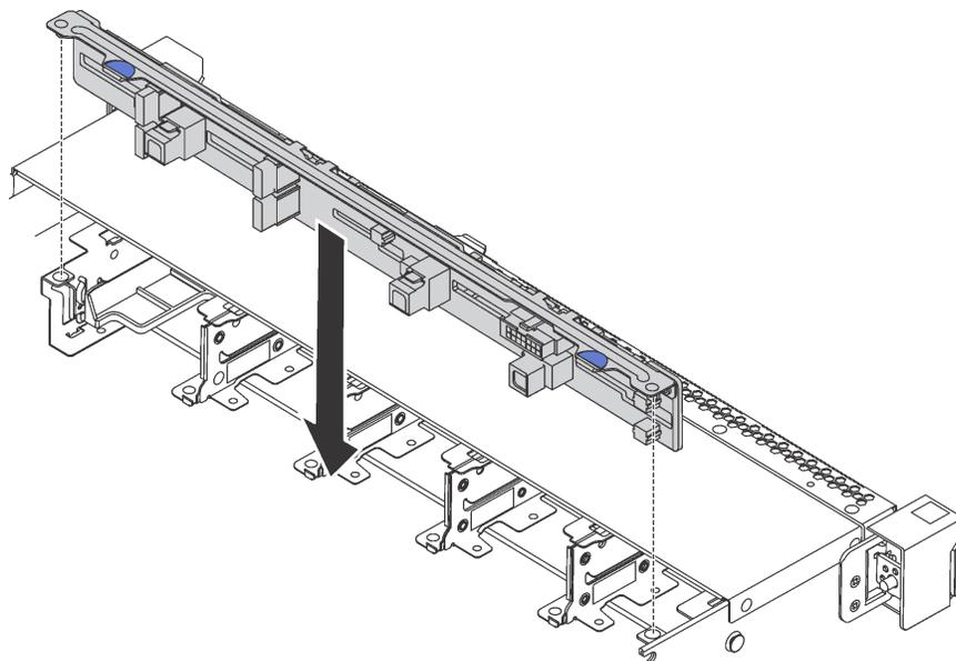
Figure 115. Installation of backplane for ten 2.5-inch hot-swap drives
