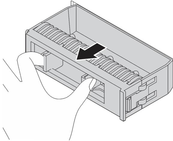
Figure 87. Drive filler removal
