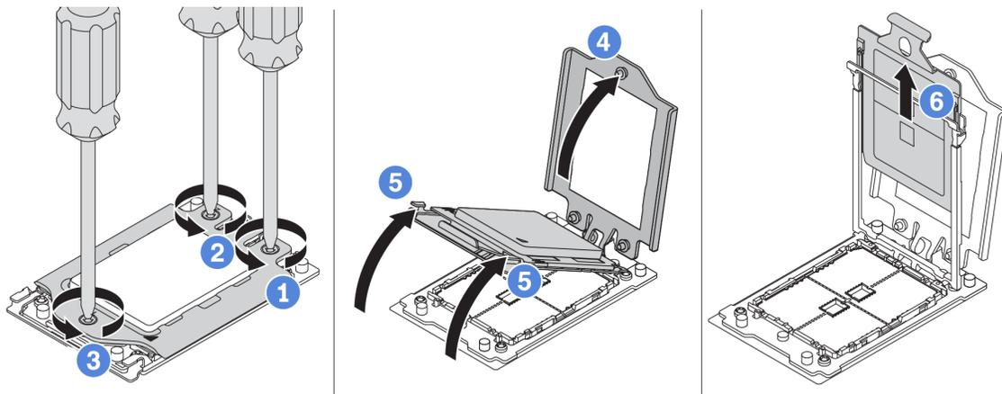
Figure 170. Removing a processor
