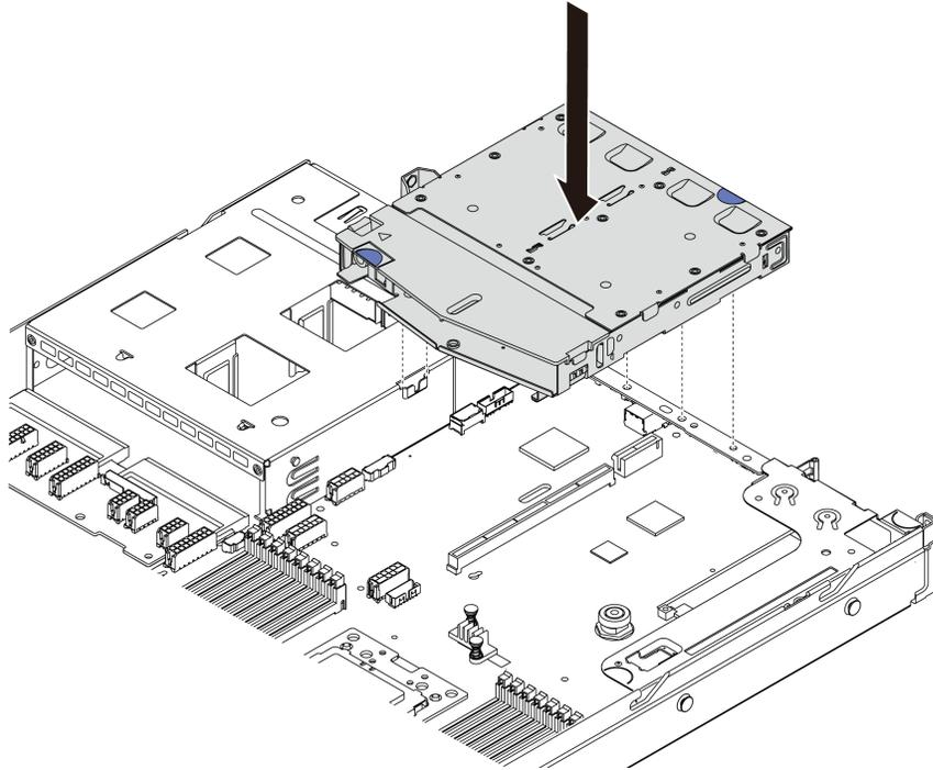
Figure 132. Rear hot-swap drive cage installation
