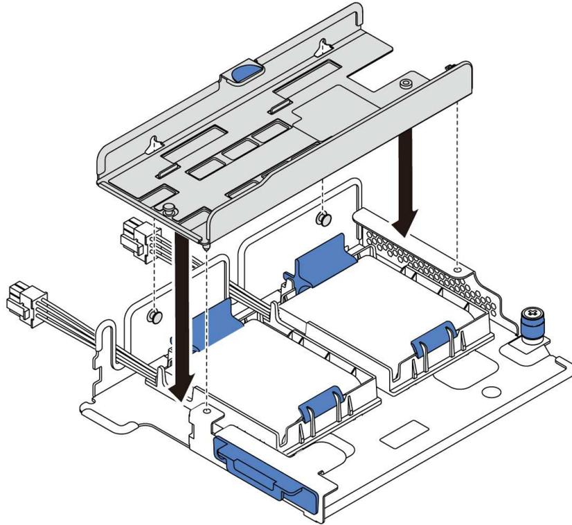
*Figure 148. M.2 module bracket installation*
