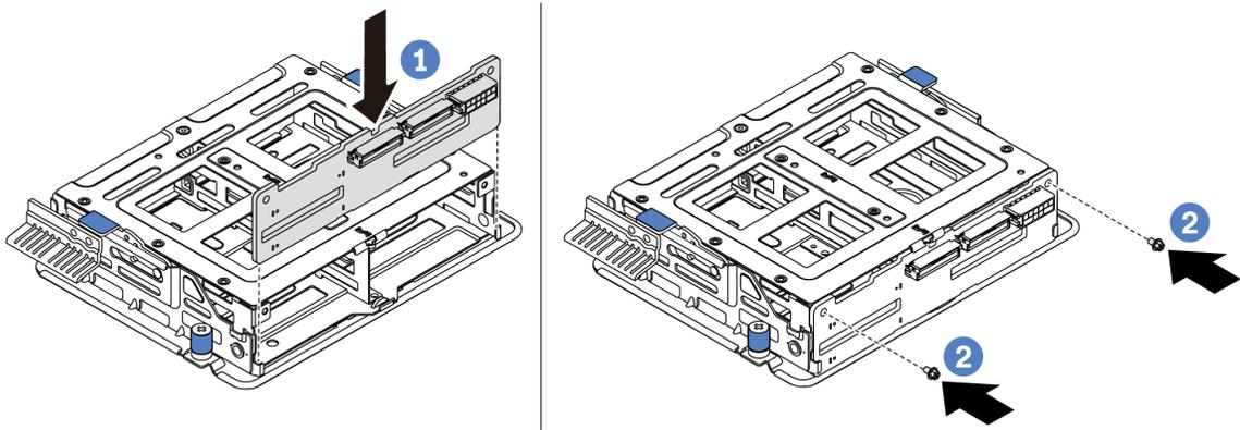
Figure 138. Internal backplane installation
