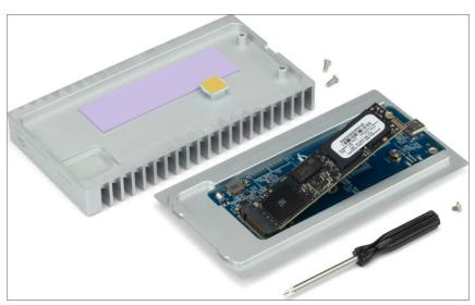
2. Once the drive is fully seated use the included drive screw to secure the drive.
