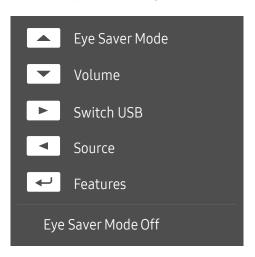
The Direct Key Guide screen shows if **Eye Saver Mode** is enabled. (**Off, Low, High**)
