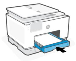
5. Insert the output tray into the printer.
