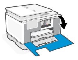
2. Open the cartridge access door, and then wait until the carriage stops moving.
