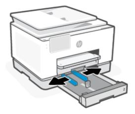
3. Press the button near the front of the tray to extend the input tray.
