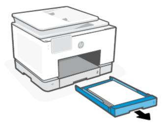
3. Check the area inside the printer where the trays were removed, and remove any jammed paper found.
