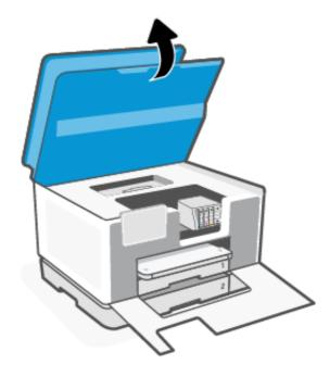
3. Look inside the printer and remove any jammed paper found. Move the carriage to the left and right to fully inspect the print area for any jammed paper.
