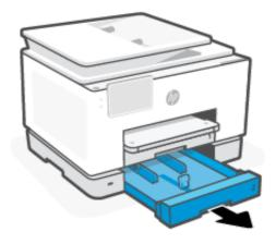
2. Press and hold the button on the paper-length guide, and then slide the guide toward the edge of the tray as far as possible.
