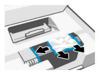
4. Lift the handle of the paper path cover and remove the cover.
