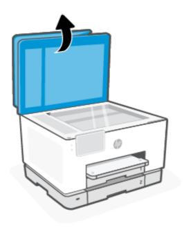
2. Clean the scanner glass and lid backing by using a soft, lint-free cloth that has been sprayed with a mild glass cleaner.
