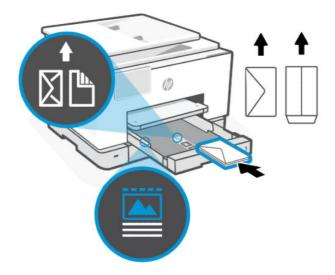
पुर्ट TIP: Use the envelope guide to load C5 and #10 envelopes with long flaps. You do not need to use the guide for envelopes with short flaps.
