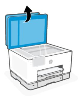
2. Load your original print-side down on the scanner glass. Align the original to the indicated corner and the engraved guides along the edges of the scanner glass.
