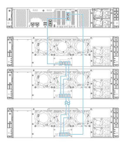
**2.** Connect the expansion units to the device using the following topology.
