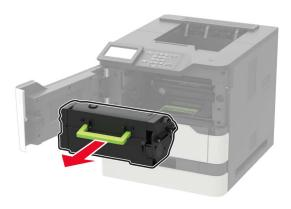
**3** Remove the used imaging unit.
