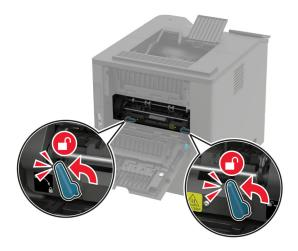
4 Remove the used hot roll fuser.
