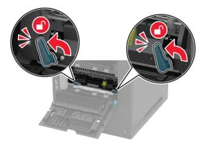
**3** Remove the used fuser.
