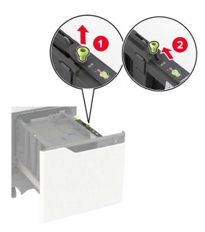
**b** If the A5 length guide is still attached, then remove it. If the guide is not attached, then proceed to <u>step</u> <u>d on page 31</u>.
