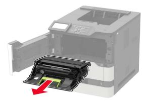
4 Remove the used transfer roller.
