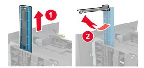
**d** Insert the guide into its designated slot, and then press until it *clicks* into place.
