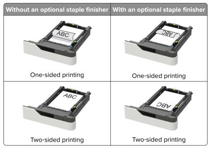
• When loading prepunched paper, make sure that the holes on the long edge of the paper are against the right side of the tray.
