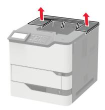
**6** Install the mailbox on the printer, and then push it down to make sure that it is securely attached to the printer.
