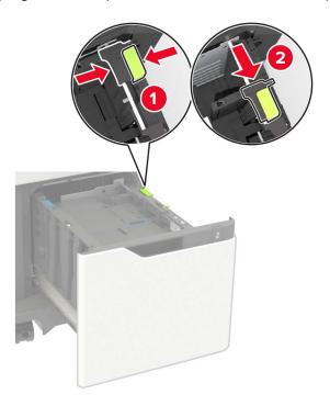
**c** Remove the A5 length guide from its holder.
