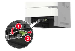
4 Using a damp, soft, lint-free cloth, wipe the pick tires.Note: Apply isopropyl alcohol to the cloth.
