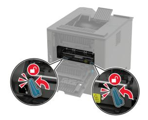
4 Remove the used hot roll fuser.
