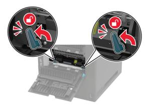
Remove the used fuser.
