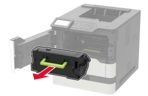
**3** Remove the used imaging unit.
