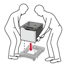
**5** Align the printer with the tray, and then lower the printer until it *clicks* into place.
