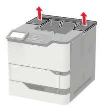
**6** Install the staple finisher on the printer, and then push it down to make sure that it is securely attached to the printer.
