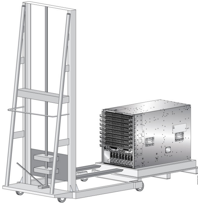
Figure 14: Align the Lifting Device in Front of the Chassis on the Pallet
