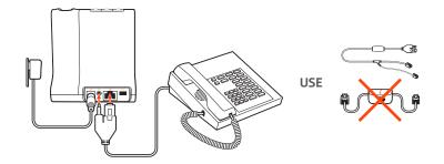
**IMPORTANT** Use configuration **A** on the bottom of the base, which works for most phones including Cisco phones.
