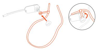
2 Choose the size and style of the eartip that fits most comfortably. Align the eartip with the notch facing the microphone as shown. Press on to attach.
