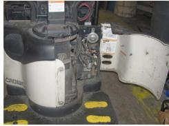
Locate the horn (shown below). Remove the horn by removing the 9/16" bolt holding it in place.
