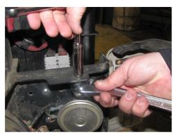
Remove the power connector bracket that is located between the battery and chasis wall by removing the four self tapping bolts that are holding it in place. On the side where the horn was previously removed, drill out the four holes that the self tapping bolts were in using a 5/16" drill bit. Using the four sets of 1/4 - 20 bolts, washers and nuts, mount the 7160-1734 bracket between the outer wall and the power connector bracket using the drilled out holes.
