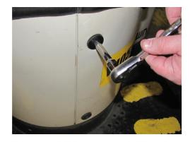
With these two bolts, removed the door should swing open.
