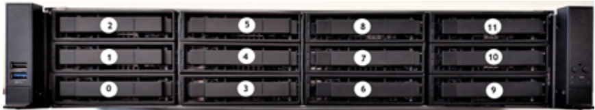
Figure 1-2 Appliance front panel drive slot assignments
