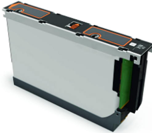
Figure 2-5 Disk Drive In Carrier (DDIC) module
