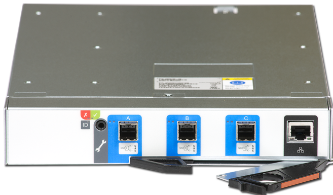
Figure 2-6 Veritas U12 65.5TiB/72TB Storage Shelf I/O module
