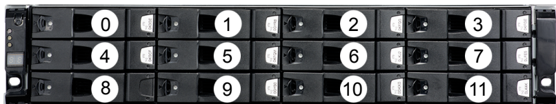
Figure 2-2 Veritas 2U12 65.5TiB/72TB Storage Shelf disk drive slot layout
