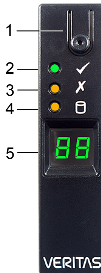
Figure 2-4 Veritas 2U12 65.5TiB/72TB Storage Shelf control panel
