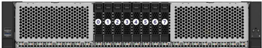
Figure 1-2 Veritas 5360 Appliance front drive assignments
