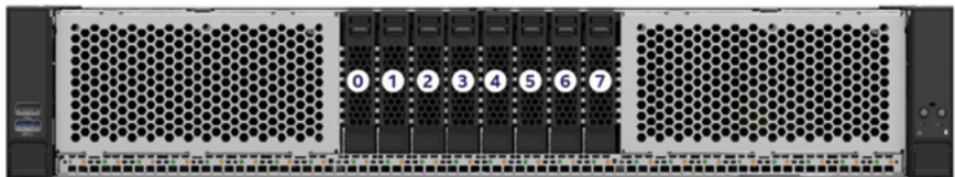
Figure 1-2 Veritas 5360 Appliance front drive assignments
