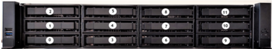
Figure 1-2 Appliance front panel drive slot assignments
