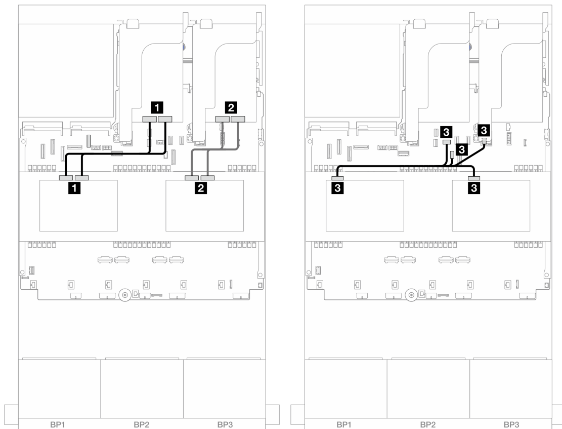
Figure 429. Middle backplane cable routing
