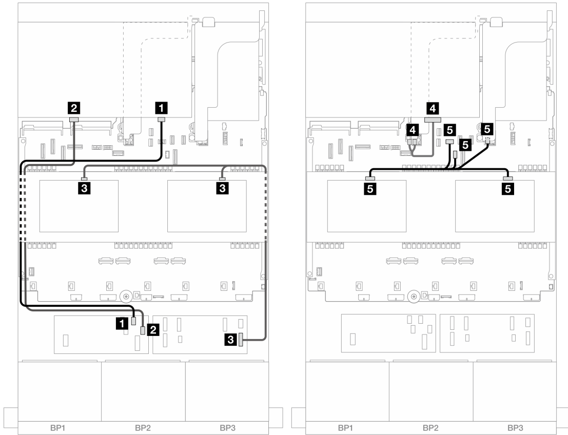
Figure 423. Middle/Rear backplane cable routing
