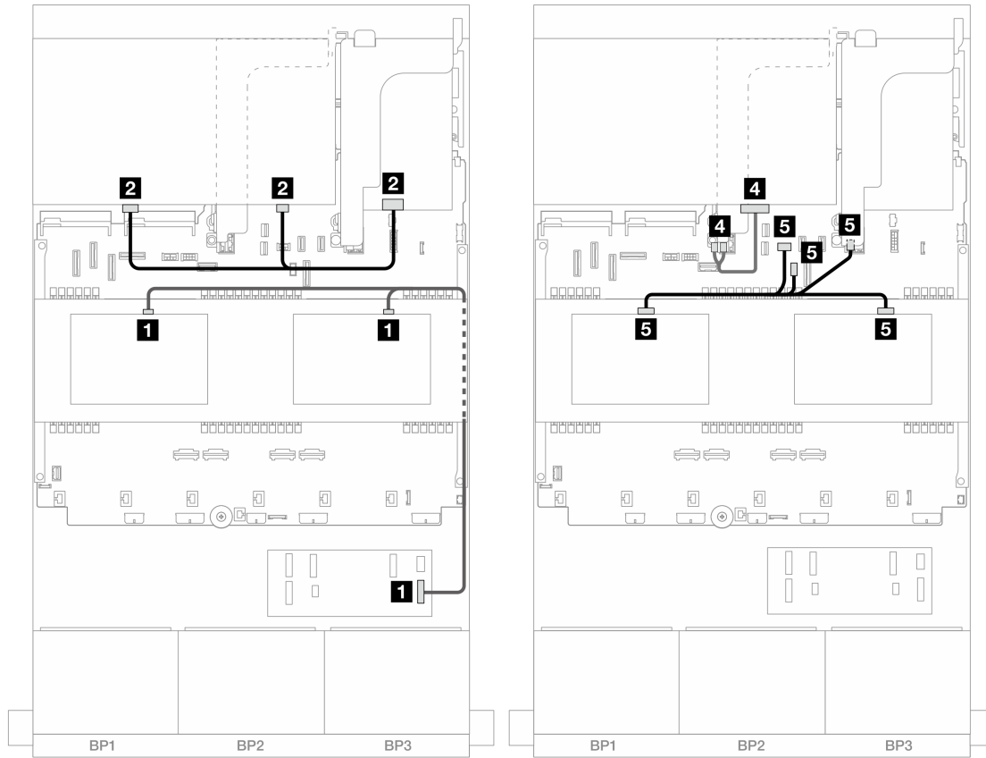
Figure 420. Middle/Rear backplane cable routing
