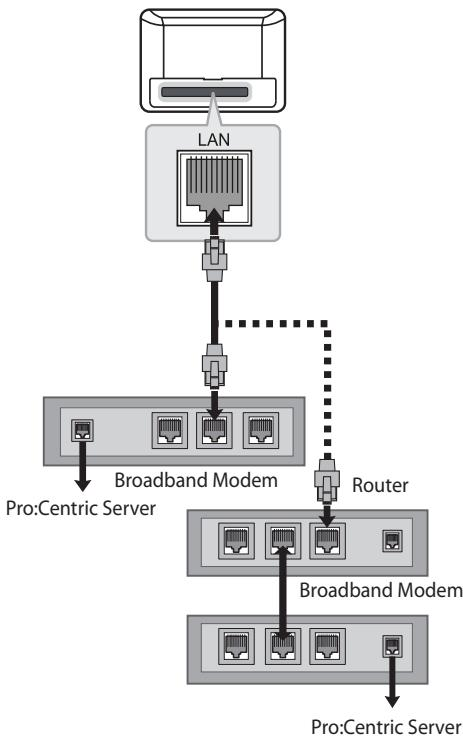
Connect the **LAN** port of the Modem or Router to the **LAN** port on the TV.
