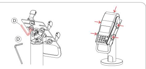
2A. Loosen connections at the rear of the holder using the included allen key tool (D). Adjust the 5 rubber clips to match your card reader device. Insert the device, and then firmly tighten the connections for a secure setup.
