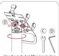
Use the included Allen key tool or wrench to loosen key joints as illustrated. Adjust to the desired tilt or swivel orientation. Securely tighten the screws for a fixed setup.
