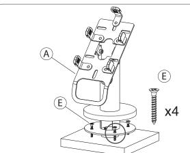
1A. Lift the canopy cover of the stand (A) to reveal the mounting plate. Align and rotate in screws (E) into surface until securely tightened. (Screwdriver not provided). Place canopy cover back on top.
