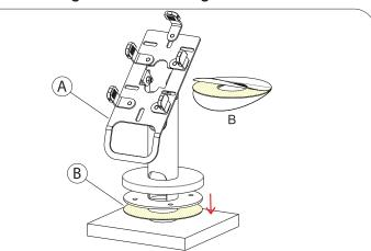
1B. Removing lining from both sides of sticker adhesive (B). Adhese one side to the bottom of the mounting plate as illustrated and the other side to the surface of the desired mounting location. Press down firmly to securely attach.
