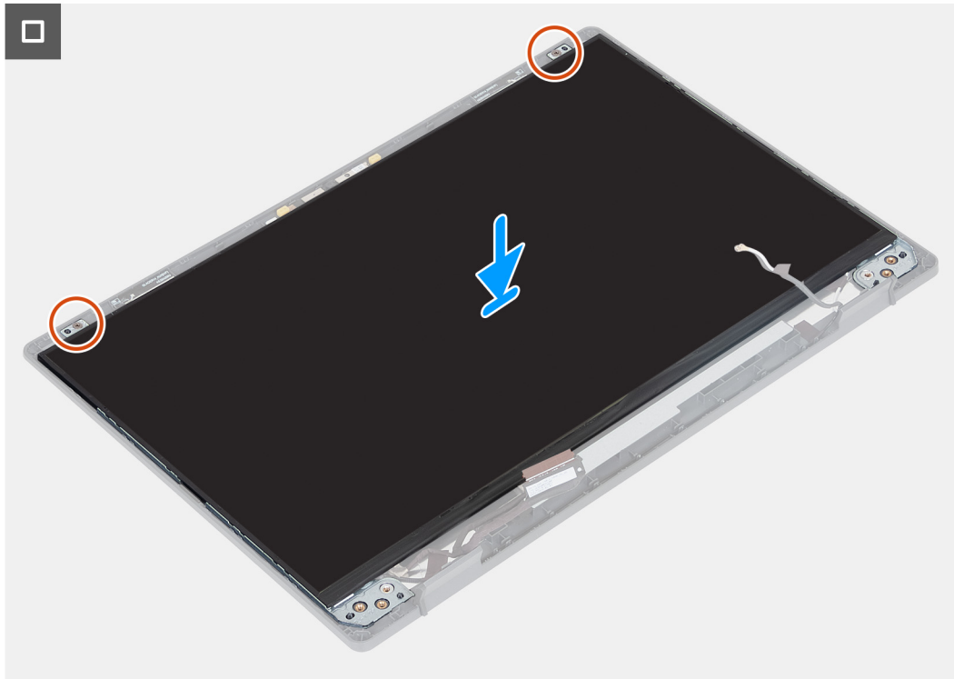
Figure 41. Installing the display panel
