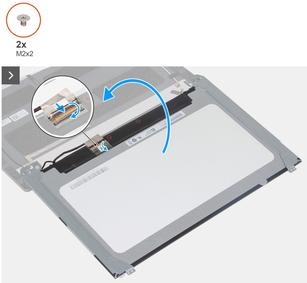
Figure 40. Installing the display panel
