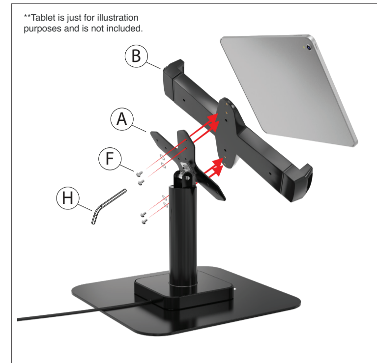
3A. Install holder (B) to VESA Base (A) by screwing in the provided screws (C) with washers (D) with the included allen key tool (H) as illustrated above.
