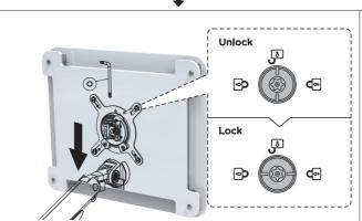
4B. Combine device with VESA plate attached with rest of clamp by sliding in at the grooves at the joint.
