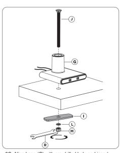
3C. Align base (G) with pre-drilled hole and insert long screw (J) through the base and hole. From below insert grommet mount components (I, L, M) onto the long screw. Using fingers initially, rotate all the grommet components until tightly fastened. Using provided wrench tool (R),rotate hex nut (M) until securely tightened.
