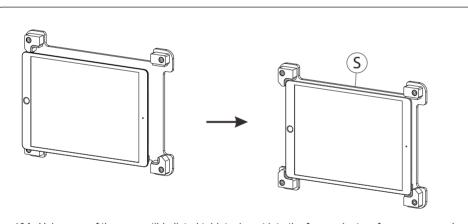
10A. Using one of the compatible listed tablets, insert into the foam adapters for a secure and tight fit.Insert tablet in back part of enclosure (S) as shown. Watch out orientation of tablet.
