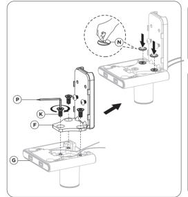
2A. Align L-shape component(F) with base of clamp mount as shown above. Rotate in screws (K) through using provided tool (P) until securely tighten. Afterwards peel off sticker back of padding (N) and place firmly on the screws
