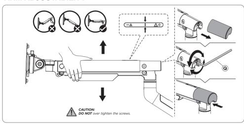
5A. To properly balance the arms with monitors mounted, adjust the spring tension using the provided allen key. Position it in the horizontal position and firmly hold the arm as shown. Tight the screw to fix it in the horizontal position.
