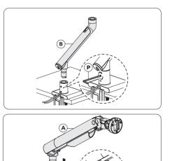
3D. Take the bottom part of the clamp arm (B) and insert the bottom connector into the base (G) as illustrated above. Then tighten with provided tool (P) until securely fastened. Then take the top part of clamp arm (A) and insert into top connector part of the bottom arm. Tighten joint with provided tool (P)
