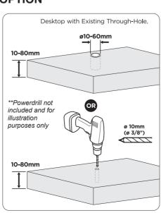
3B. Using drill (not included), drill a 10mm diameter hole for the grommet mount installation. If existing hole is available, make sure diameter is in the 10-60mm range prior to setup for proper installation.
