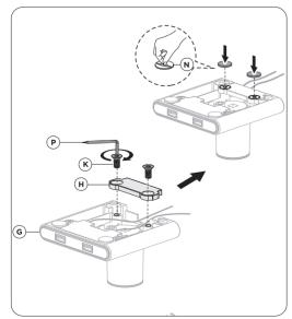
3A. Align base (G) with component (H). Rotate in screws (K) with provided tool (P) until securely tightened. After, locate base pads and remove backing. Place adhesive side of pads
