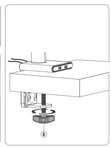
2C. Rotate knob (E) until securely tighten to
