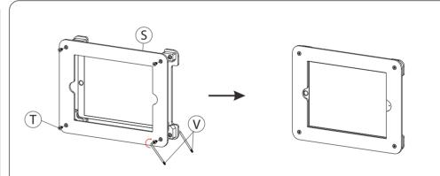
11A. Take the detached enclosure top (S), align the corner holes with the bottom portion. Then use the provided security star key (V), turn in clock-wise the star screws (T and U) until securely tightened while holding the security star key (V) on the other side with your other hand. Screw in until securely tightened.
