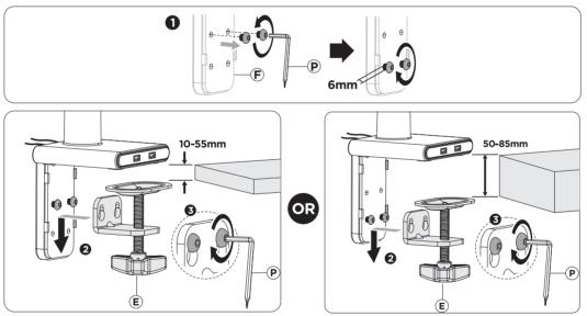
2B. Identify the overall thickness of the surface the clamp will be mounting on. If the thickness is in the 10-55mm range, you will be using the higher setting on the L-shape bracket of the base. If the thickness is in the 50-85mm range, you will be using the lower setting. Rotate in the screws (F) of the bracket until halfway in leaving some space. Hook on the knob component (E). After hooked on, use the provided tool (P) and securely tighten the screws (F) until securely fastened
