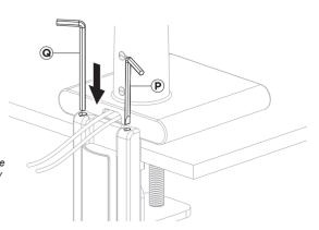
8A. When fully finished with setup, place the provided tools (Q, P) in the tool organizer (F) as shown for easy clamp angle and orientation adjustments when needed.
