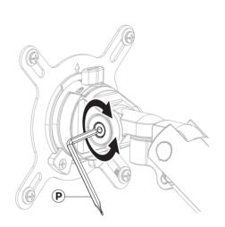
7A. Loosen the joint (as shown) behind the VESA plate using provided tool (P). When loose, tilt up and down or rotate portrait / landscape for preferred viewing angles and setup. When done, tighten screw again until securely fastened.
