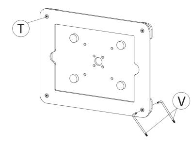
9A. Align the security star keys x2 (V) and insert it one in the front screw (T) and one in the Back screw (U) as shown.
