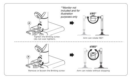
5C. When making swivel adjustments to the arm, use provided tool (P) at the joint above the mount as shown above. Loosen to allow for swivel rotation as shown. Then rotate clockwise to tighten again once desired rotation has been set for preferred setup.
