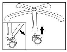
Screw wheels into floor base by hand, then use wrench to tighten.
