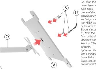
now dissembled back (U) piece of the enclosure (V) and align it with the VESA plate of the arm (O). Screw the bolts (S) from the front using the included allen key tool (U) until securely tightened. Thearm's holes are threaded so no back hex nuts are required.
