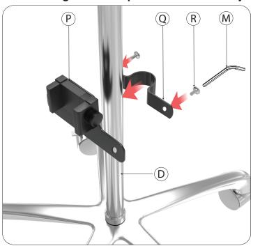
5A. Find the power strip holder component and first remove the screws with provided tool (M). Take the two halves (P+Q) and wrap them around the body pole as illustrated above. Using the provided tool (M), rotate the screw until securely tightened. No hex nuts are needed because the holder is threaded and will hold the tightened screw.
