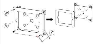
7A. Align the (2) security star keys (Y) and insert them through the front and back. While holding the back one, turn the front one (D) counter clock-wise until all (4) screws (W) are unscrewed. Separate front part of enclosure (V) as shown.
