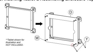
9A. Insert the compatible tablet into the opened enclosure for a secure fit as shown. Take the detached enclosure top (V), and align the corner holes with the bottom portion. Use one of the provided security star key (D), and turn in clock-wise the until securely tightened while holding the 2nd security star key (D) on the other side with your other hand. Screw in until securely tightened.
