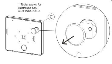
6A. When installing device into the enclosure, identify where the camera is. Then simply remove and pop out the cover prior to mounting or setting up tablet to properly expose camera.
