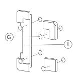
4A. Identify the double sided adhesives (G). Peel away the backing on both sides. Adhesive four of them behind the foam pieces (I) as illustrated. They are to adhese the foam to the enclosure. Peel away the back on the next four and place them on top of the foam pieces as illustrated. These are to attach the foam to the tablets and ensure
