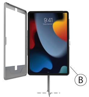
3B. Place the tablet device in the Enclosure (B)
