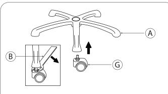
1A. Take one wheel (G) and align it to the leg arm holes on the underneath of the base (A). Initially you can use your hands and manually rotate the wheel until slightly tightened. Then use the provided wrench tool (B) at the hex shaped area and rotate it securely to tighten the rest of the way.
