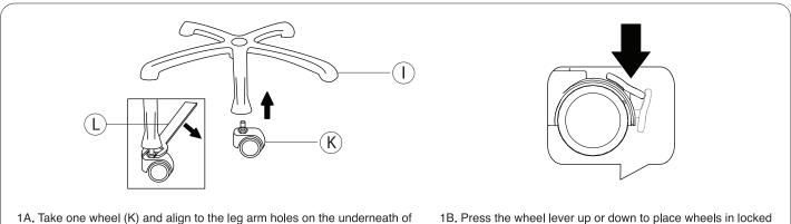
the base (I). Initially you can use your hands and manually rotate the wheel until slightly tightened. Then use the provided wrench tool (L) at the hex nut and rotate to securely tighten the rest of the way. As shown above.
