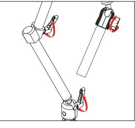
2. Adjust the arm to your preferred position and then tighten the screw knob clockwise.
