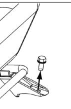
2.Install the assembled Vechicle Seat Rail Clamp and Base set on the seat rail and screw back the bolt.
