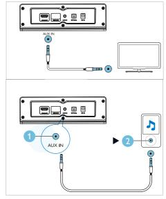
Using a 3.5mm stereo audio cable, connect the AUX IN connector on your SoundBar to the AUX connector on the TV or other device.
