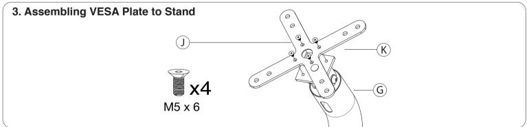
3A. Align the VESA plate (K) holes to curved swan neck (G) holes. Then insert the (4) screws (J) and rotate in with the provided tool (M) until securely tightened.
