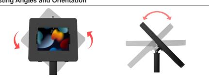
Tilt up/down for preferred angles as needed. Rotate left and right for preferred orientation.
