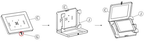
3A. Lock or unlock your tablet enclosure (C) with security key (G) as shown.
