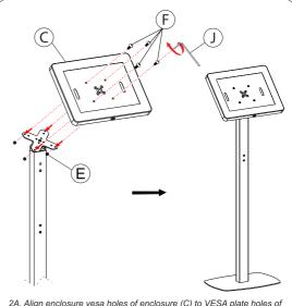
2A. Align enclosure vesa holes of enclosure (C) to VESA plate holes of floor stand (A). Rotate in screws (F) using provided tool (J) while holding hex nut (E) from behind with fingers.
