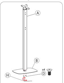
1A. Align the base plate (B) with floor stand body (A) and rotate in the screws(D) from below with the allen key (H) until securely tightened.
