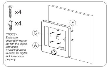
1A. Align the enclosure to the wall and mark off the holes with a pencil (not included). Use a drill (not included) and predrill locations. Insert (4) anchors (E) as illustrated into the wall drilled holes. Then align VESA holes of enclosure and rotate in screws(G) until securely fastened.
