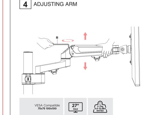
To properly balance the arm with monitors mounted, adjust the spring tension using the supplied Allen Key as follows:
