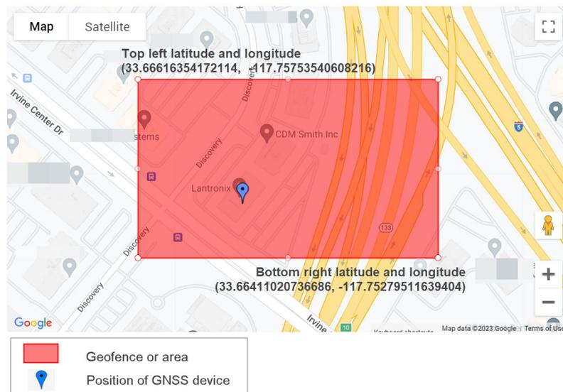
An Area is composed of up to 100 geofences. The geofences may be overlapping or not. [Figure 18-2](#) shows an example of a geographic area composed of overlapping rectangular geofences. Entry and exit events occur when the GNSS-equipped device enters or exits the area, respectively.
