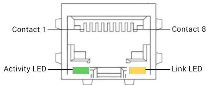
Table 2-8 Ethernet RJ45 Connector Pin Assignment and LEDs
