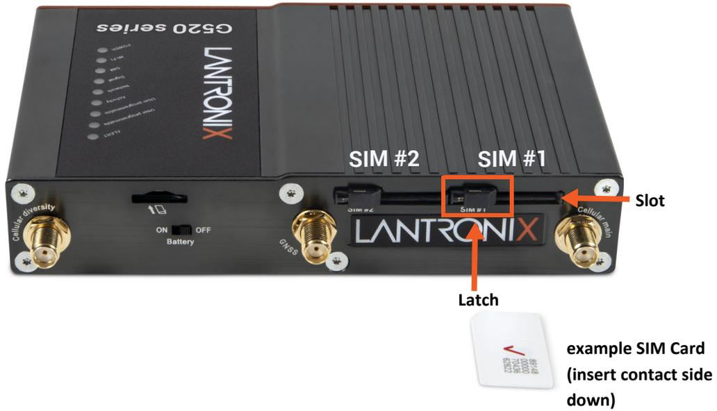
2. Gently insert the SIM card (contact side down) into the slot and push to lock it in place. Release the latch.
