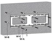
1.2B: Place the anchors (W-B) into the wall, and then align the 4 washers and screws (W-C, W-A) to the pre-drilled holes. Using a socket wrech tool (Not included), rotate in the screws until securely tightened.
