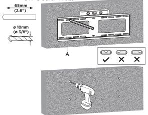
1.2A: Place the wall bracket (A) on the desired location on the wall and with a level (not included), mark off the location of the drill points as illustrated above. Afterwards use a powerdrill (not included) with a 2.6" length and a 3/8" diameter drill bit, and drill where was marked
