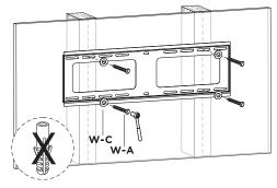
1.1B: While holding the wall bracket (A), align the 4 washers and screws (W-C, W-A) to the pre-drilled holes. Using a socket wrech tool (Not included), rotate in the screws until securely tightened.
