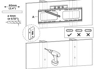
1.1A: Identify the wall studs and locate where you want to place your mount. Place the wall bracket (A) on the wall and with a level (not included), mark off the location of the drill points as illustrated above. Key point is to align any of the holes to the spacing of the studs. Afterwards use a powerdrill (not included) with a 2.4" length and a 5/32" diameter drill bit, and drill where was marked.
