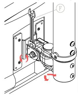
Turn bolt with wrench (F) to loosen connection, allowing adjusting ease of tilting in the VESA plate. Turn it clockwise to tighten the connection.
