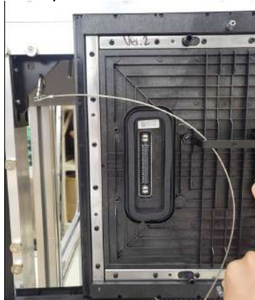
(1) Safety ring fastened during module disassembly
