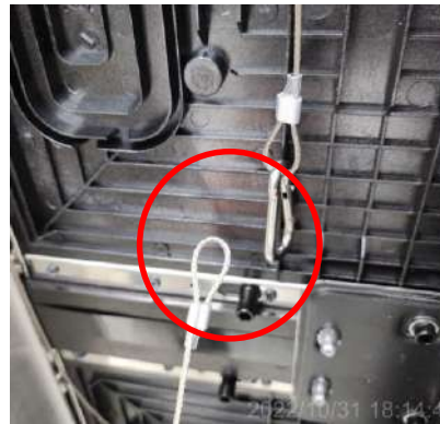
(2) Release the safety hook and release the safety wire from the module handle
