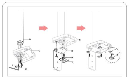
1AA. Rotate in the (3) screws (L) through the base (C) and pole (B) using the allen key tool (Q). Then, rotate in the (3) screws (M) through the component (D) and base (C). At last, adhere the (4) rubber pads (O) to the base (C) as shown by removing the covers.
