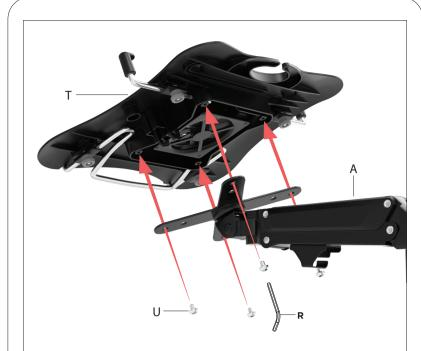
3B. Install the laptop holder (T) to VESA plate (A) by aligning the holes and rotating in the provided screws (U) using the included allen key tool (H) as shown above.
