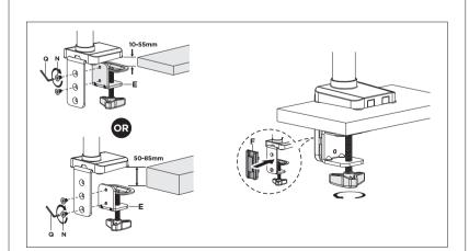
1AB. If clamping to a 10-55mm surface, rotate in the (2) screws (N) in the top holes of component (D) using the allen key tool (Q). If clamping to a 50-85mm surface, rotate in the (2) screws (N) in the bottom holes of component (D) using the allen key tool (Q). At last, attach the tool holder (F) to component (E) from the back to cover the holes as shown above.
