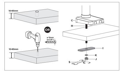
1BB. Use a pre-dilled surface or drill a hole on the surface as shown above. Insert the grommet component (H) inside the hole. Then, insert through the rod the component (I), then the washer (K) and at last the hex nut (J), and use the included wrench (S) to securely tighten the assembly to the desired surface.
