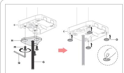
1BA. Rotate in the (3) screws (M) through the grommet component (H) and base (C) using the allen key tool (Q). Then, adhere the (4) rubber pads (O) to the base (C) as shown by removing the covers.
