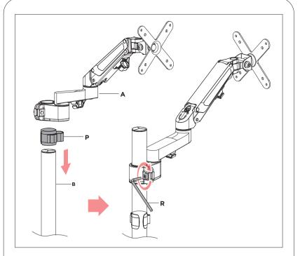
3A. Insert component (P) and (A) through the pole (B). Once in the desired position, rotate the hex screw on component (A) base using the included allen key tool (R) until securely tightened.
